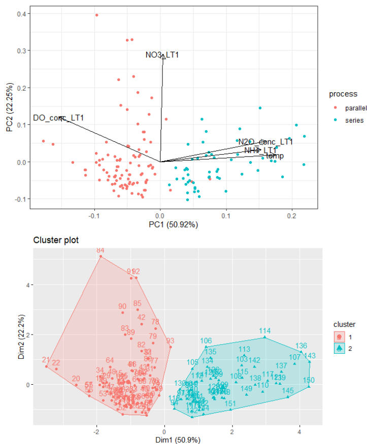
Figure 9. Principal component analysis of the main variables: ammonia concentration, nitrous oxide concentration, dissolved oxygen concentration and nitrate concentration. The different colors correspond to the two different periods of operation. And cluster plot using the k-means clustering method.
