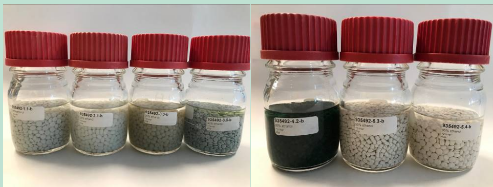
FIGURE 21 Image of samples immediately after migration to 95% ethanol. From left to right, the samples are numbered 1.1, 2.1, 3.3, 3.5, 4.2, 5.3, and 5.4. No swelling is observed.
