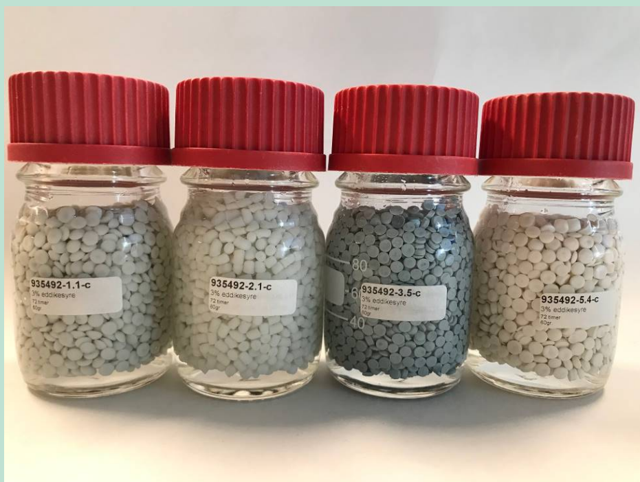
FIGURE 23 Image of samples immediately after migration to 3% acetic acid. No difference in the material is observed after migration. Note that the material floats on top, as the density of this migration liquid exceeds the density of the sample material.
