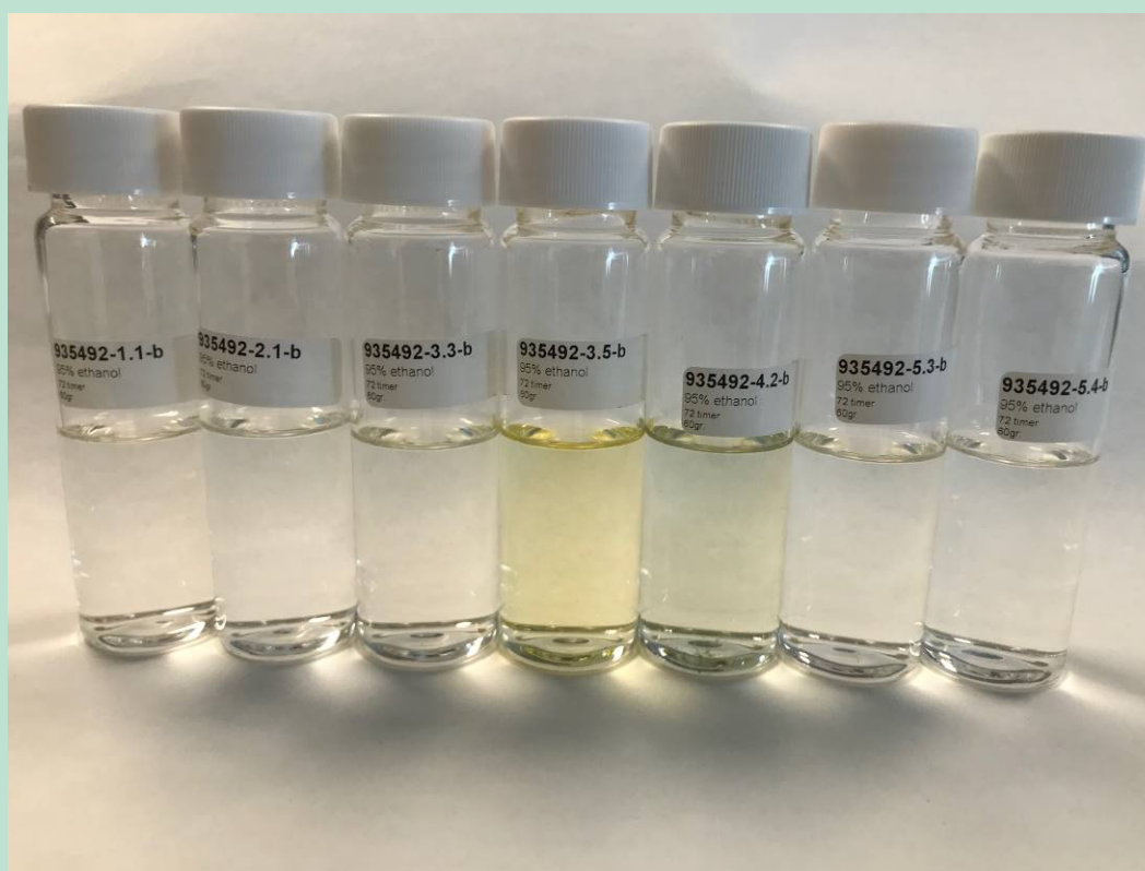
FIGURE 22 Image shows the migration liquid - 95% ethanol extracted after migration. It is visible that some samples have acquired color from the migration. This applies to samples 3.5 and 4.2. No unclear phases are visible in sample 5.3 as observed when using isooctane.
