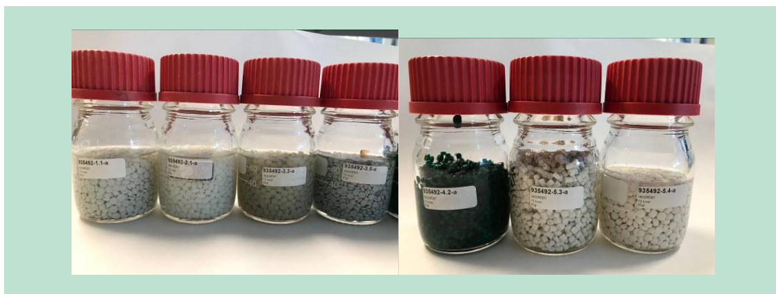
FIGURE 19. Image of samples immediately after migration to isooctane. From left to right, the samples are numbered 1.1, 2.1, 3.3, 3.5, 4.2, 5.3, and 5.4. It is visible that samples 4.2 and 5.3 have absorbed migratory liquid and are swollen.
