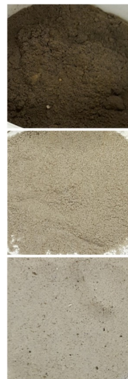
FIGURE 5: Visual appearance of untreated sand (top), after attrition cell (middle), and full MOPS treatment (bottom)
