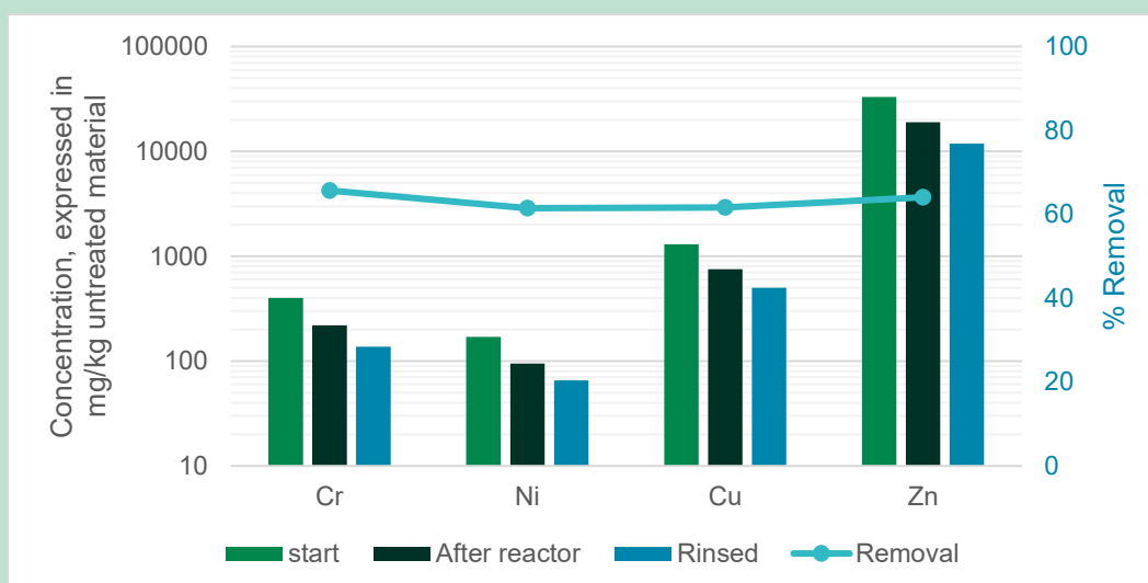
FIGURE 12. Concentrations of selected metals in untreated alkaline ash (start), after reactor and after conditioning, given as log mg/kg DM. Calculated percentage removal rates on secondary y-axis
