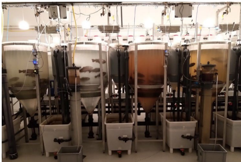
FIGURE 6.4.3. Effect of the different treatments on water clarity. From left to right: Ozone, Ozone + foam fractionator, control and finally foam fractionator.
