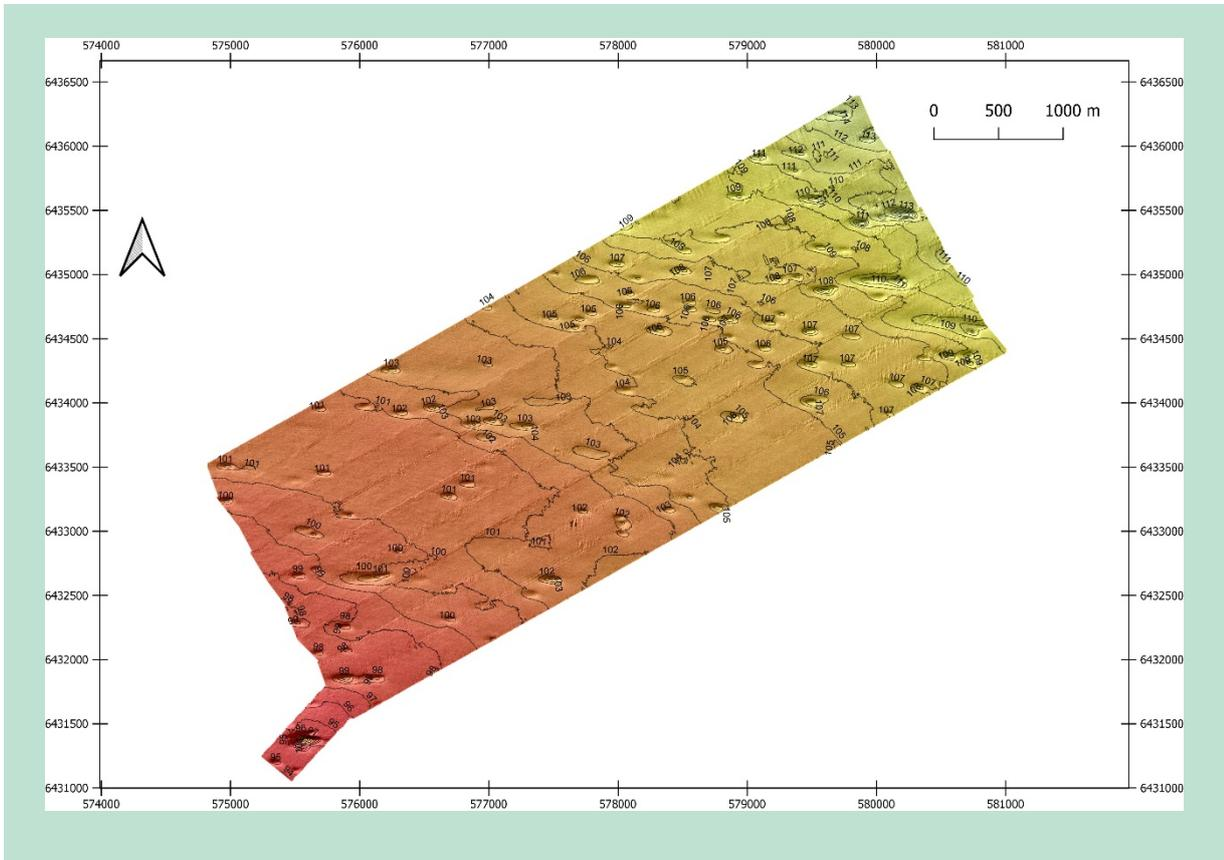
**FIGURE 6.** Bathymetry acquired in 'Area 1', where 103 pockmarks were identified following the survey.
