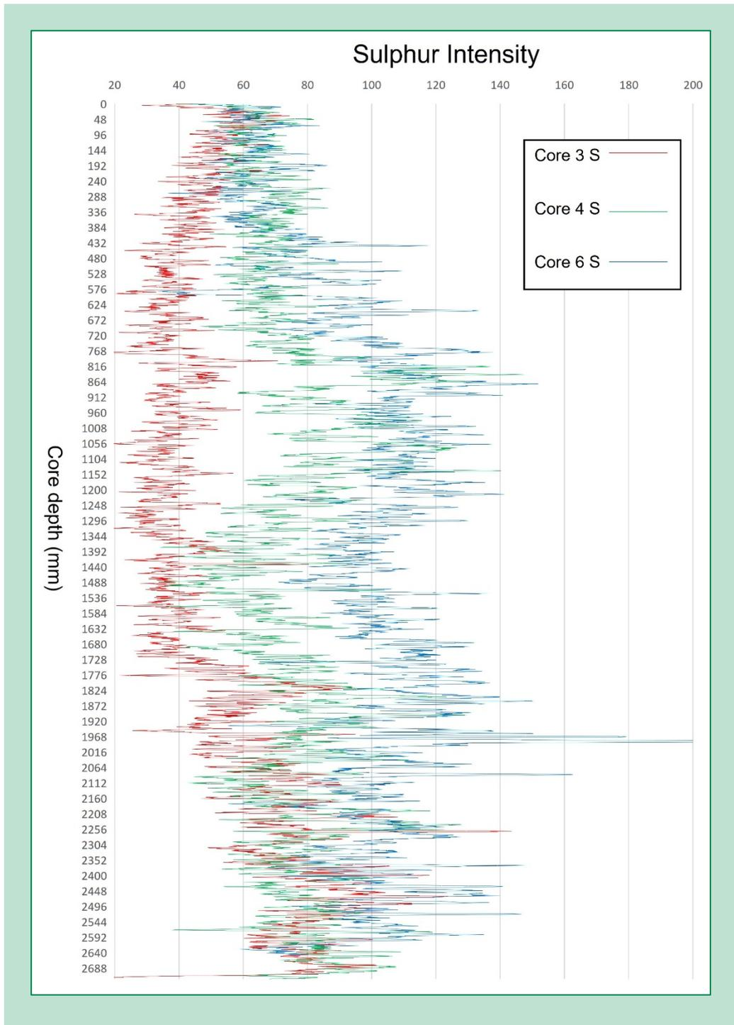
**FIGURE 13.** Sulphur content (Intensity measurement) for Cores 3, 4 and 6.
