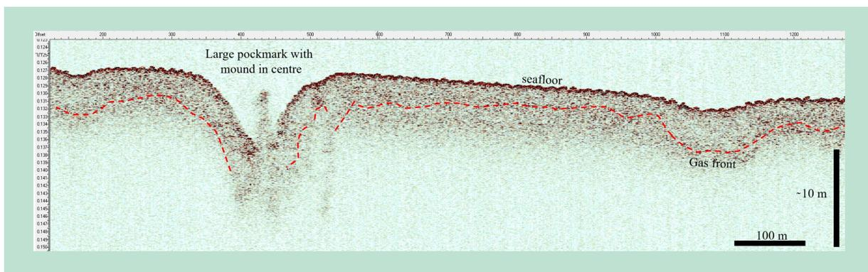
**FIGURE 16.** Subbottom profiler line from 2020 across the large pockmark and mound within area 1 (13 x vertical exaggeration).
