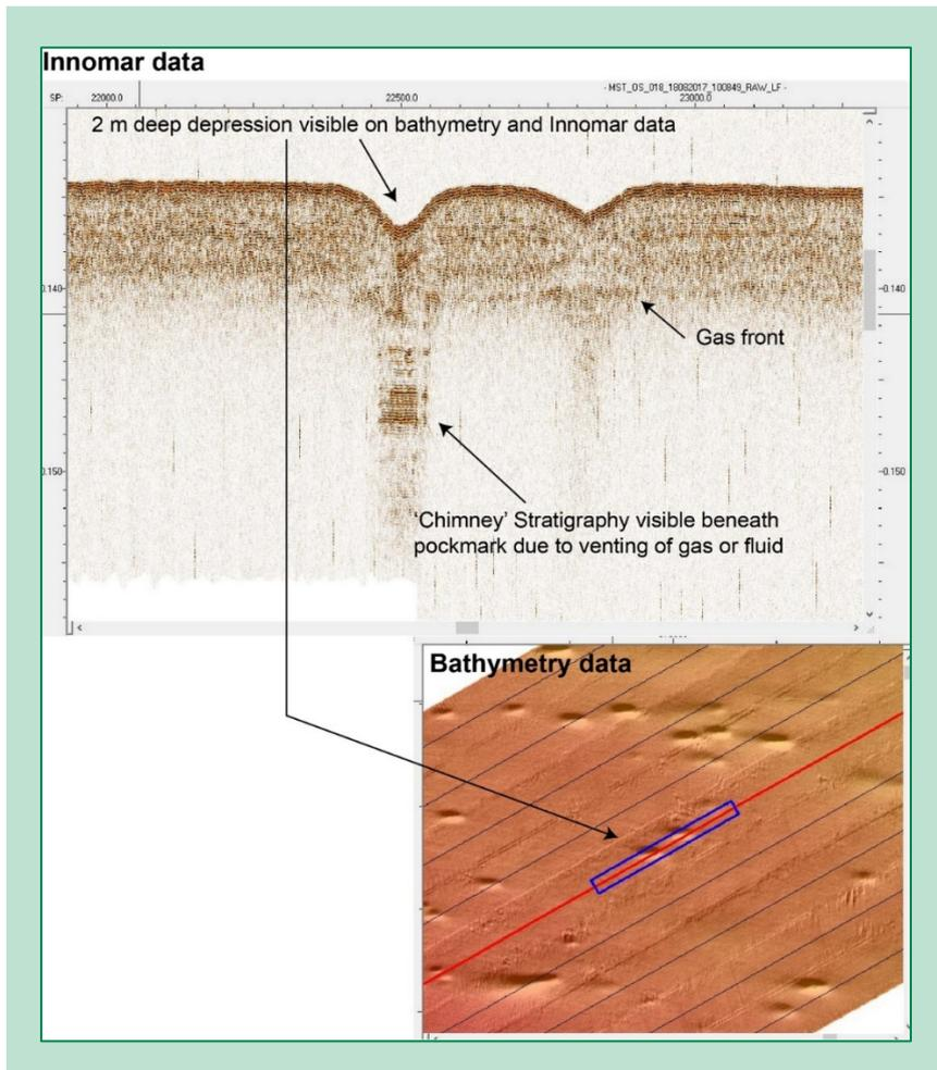
**FIGURE 4.** Example of identified pockmark with sub-surface 'Chimney'.
