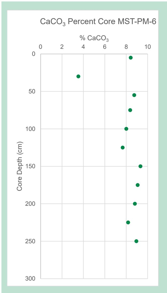
**FIGURE 10.** Carbonate percentages for core 6 (within larger complex pockmark). Following a delay, caused by the shut-down of the Aarhus University Geoscience Laboratory during the COVID19 outbreak, core PM-6 was also analysed for carbonate content. The results of this analysis are shown in Figure 10.
