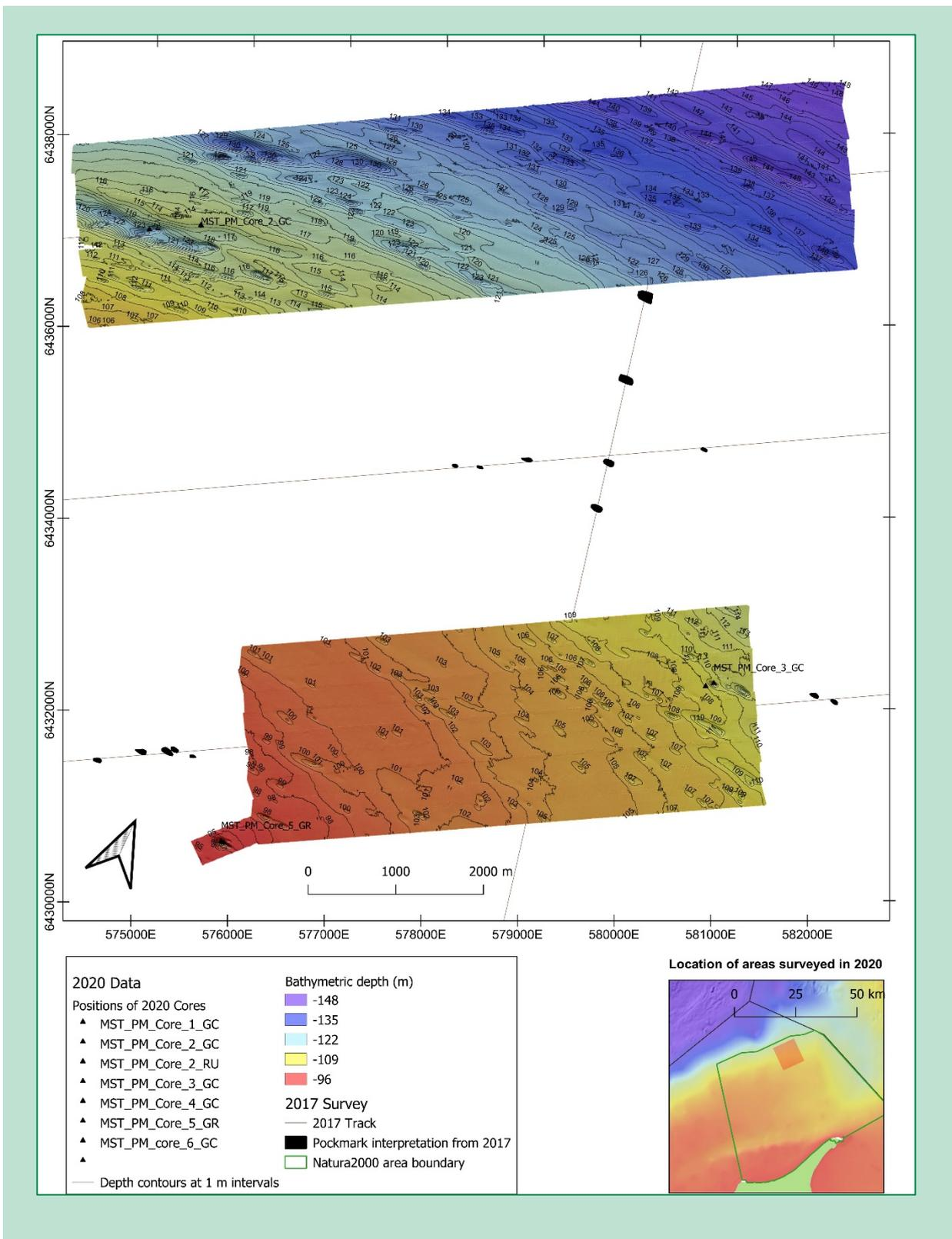
**FIGURE 5.** Overview of newly acquired data, with respect to the 2017 track plot and pockmarks identified during that year's survey.
