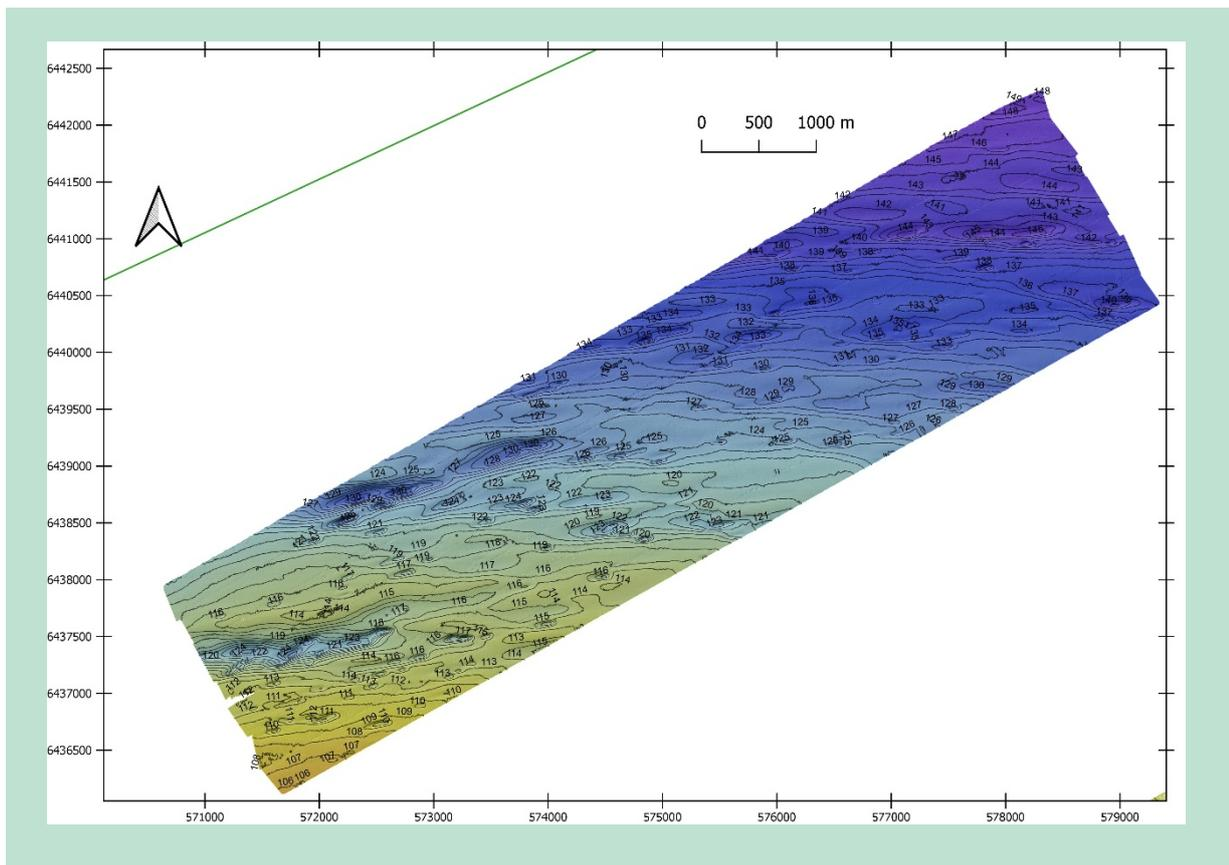
**FIGURE 7.** Bathymetry acquired in the deeper water 'Area 2', where 123 pockmarks have been identified.
