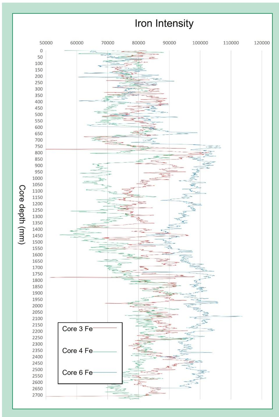
**FIGURE 12.** Iron content (Intensity measurement) for Cores 3, 4 and 6.
