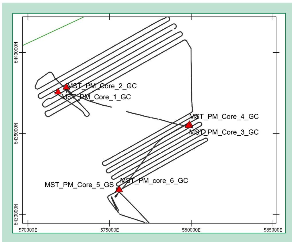
**FIGURE 3.** Track from the survey activity and location of cores. GC indicates gravity cores while GS indicates the grab sample
