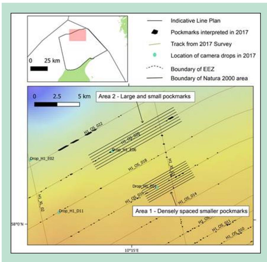
**FIGURE 1.** Location of area of interest within the Skagerrak Natura2000 area. Main panel shows the proposed survey line plan with the 2017 survey track and pockmark interpretation shown.
