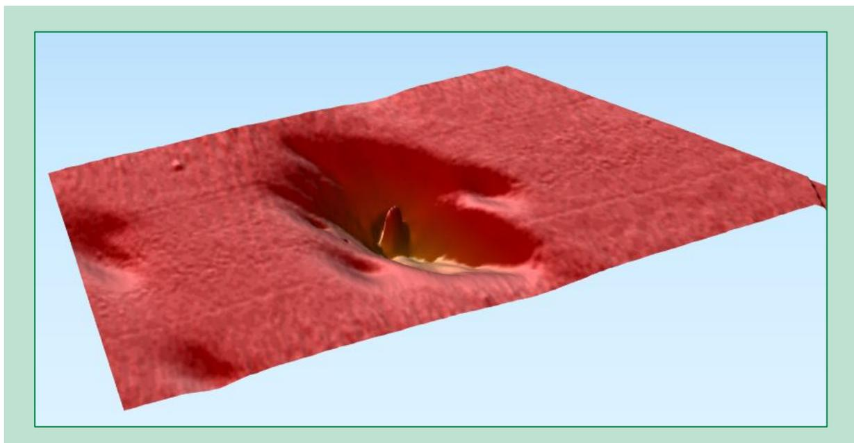
**FIGURE 15.** 3D image of large pockmark and mound within area 1 (10 x vertical exaggeration).
