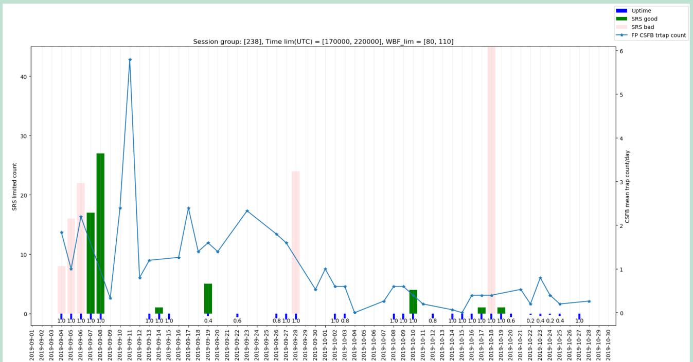
**FIGURE 8** A comparison between the cabbage stem flea beetle count per day as classified by the simple wing beat frequency and time restricted classifier for the first FaunaPhotonics prototype sensor (denoted SRS in the Figure legend), compared with the mean cabbage stem flea beetle count per day in the FaunaPhotonics water traps.
