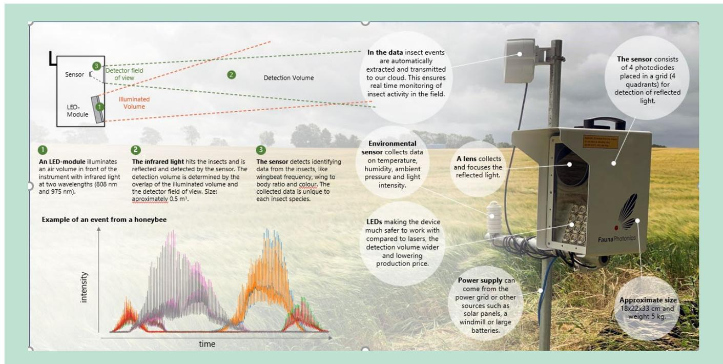
**FIGURE 1.** A schematic view with explanatory text on the FaunaPhotonics sensor, the Volito
