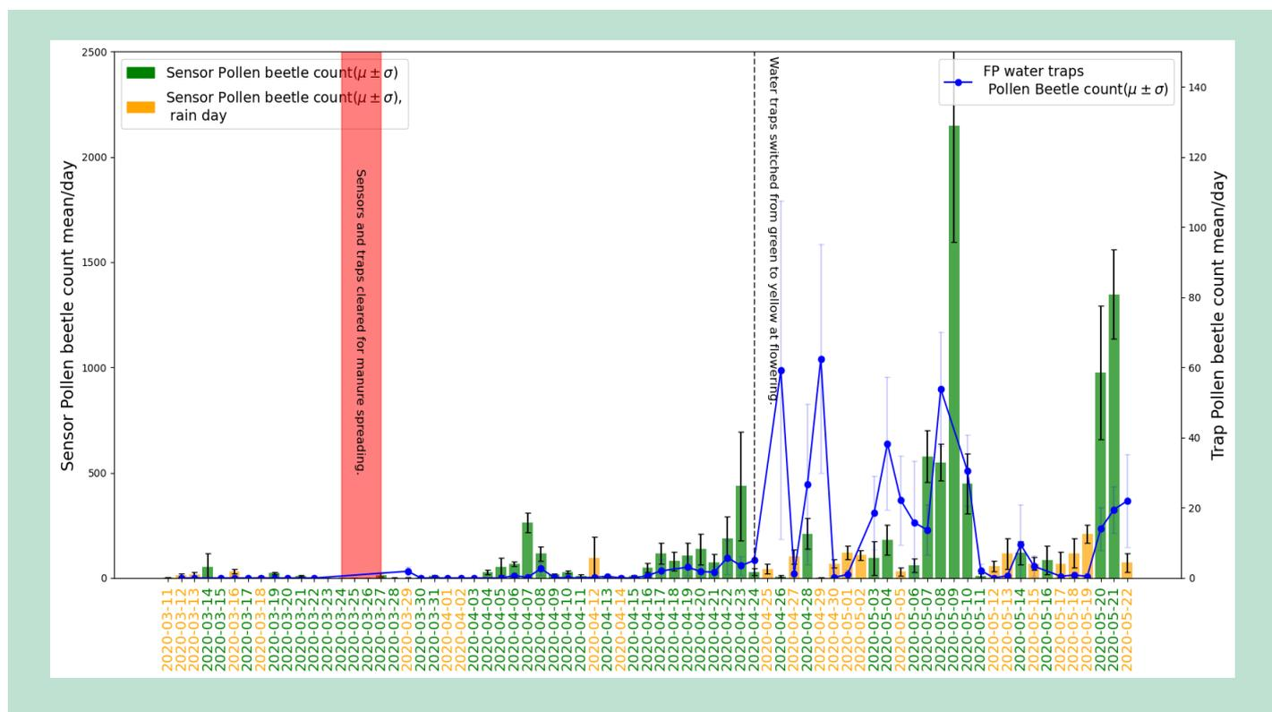
**FIGURE 10** Mean pollen beetle count per day from six FaunaPhotonics Volito sensors based on a trained pollen beetle classifier, compared with the mean pollen beetle count per day for six adjacent FaunaPhotonics water traps.
