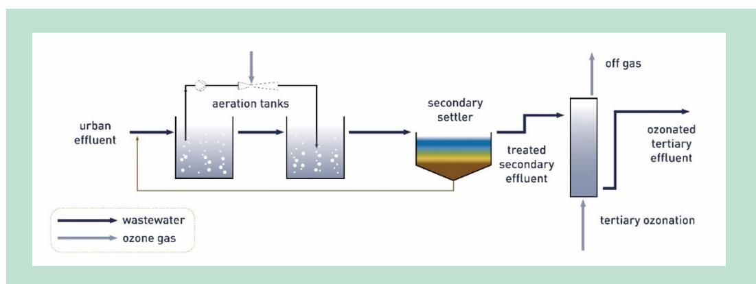
**FIGURE 8.** Schematic drawing of the experimental layout in Brødstrup WWTP.
