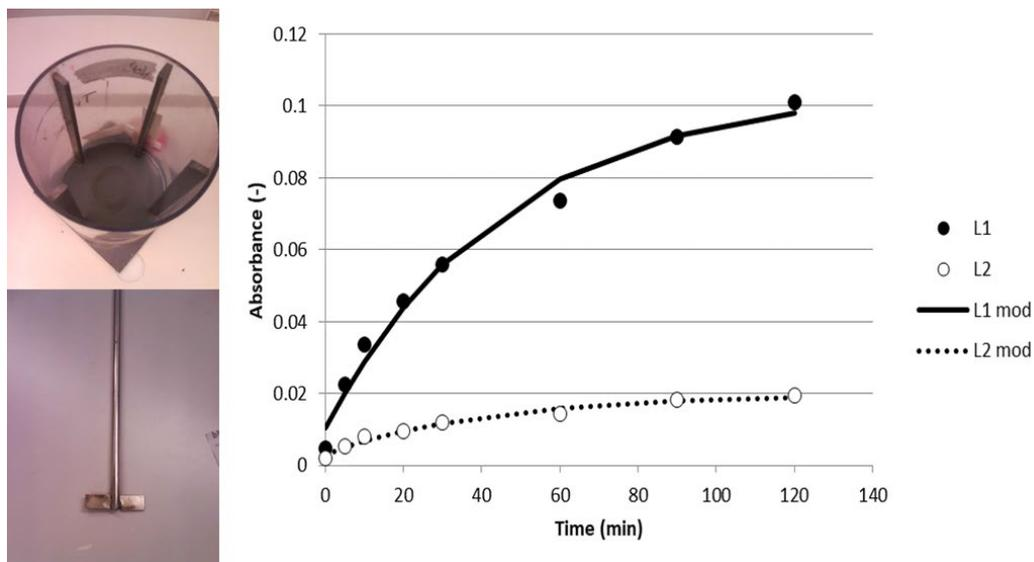
Figure A1.3: Baffle reactor and paddle for deflocculation (left) and measured development in residual turbidity over time during deflocculation by shearing (right) measured in Line 1 (L1, ●) and Line 2 (L2, ○).
