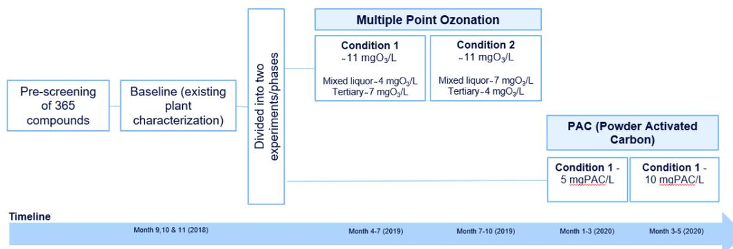
Figure 1 Schematic representation of the experimental programme. Also shown are the specific dosages of both ozone and Powder Activated Carbon (PAC). Please note that ozone and PAC never is dosed simultaneously.
