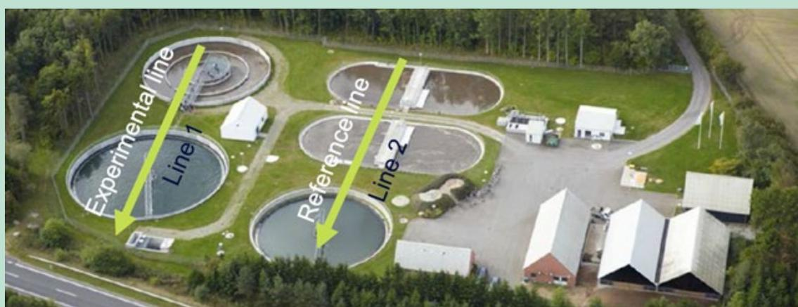
**FIGURE 1.** Show Brødstrup WWTP. The experimental line and reference line split in the outlet of the sand- and grease trap.
