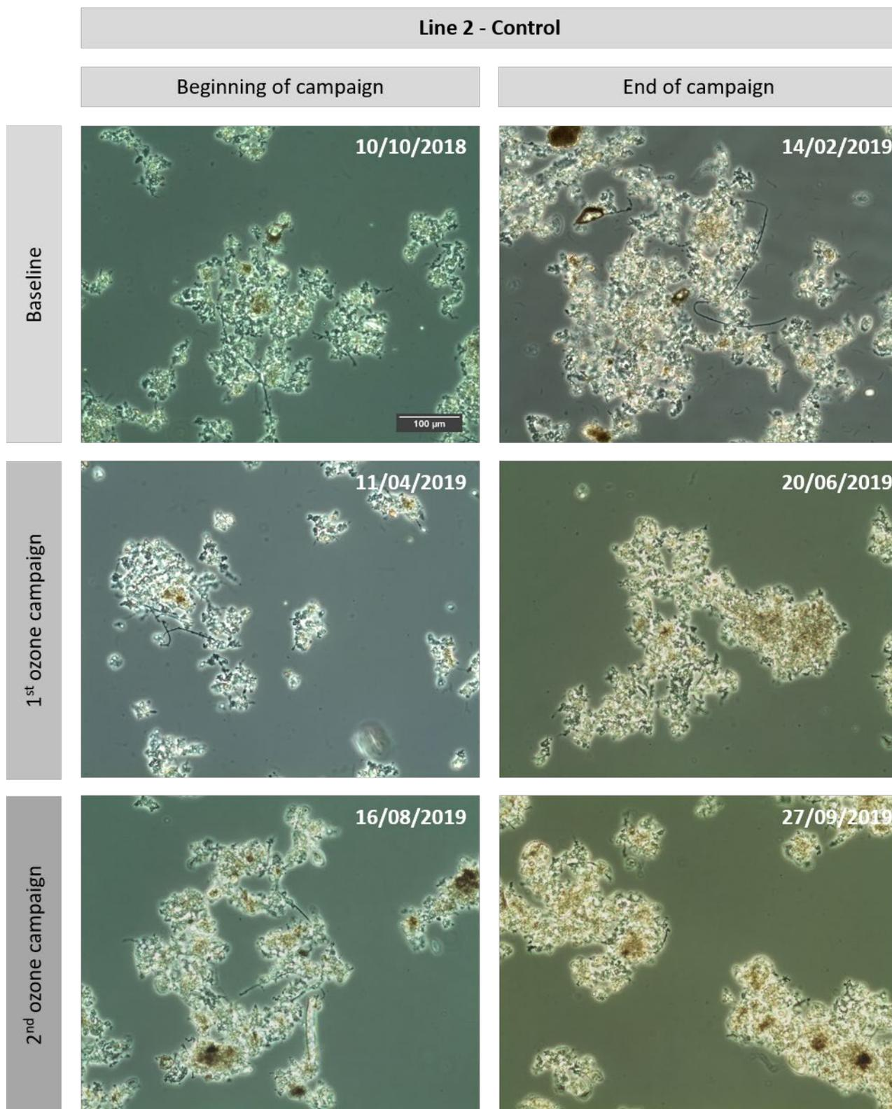
Figure 6 - Microscopic observation from Line2 - "Control". Development of floc structures during conditions in the control line.
