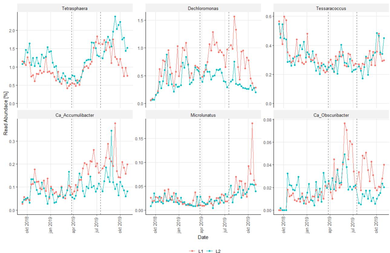
Figure 14 - Time series of known PAOs in line 1 – experimental (red) and line 2 - control (blue). The dotted vertical lines represent the start of the two ozone conditions. Note the Y-axis varies in the figures.
