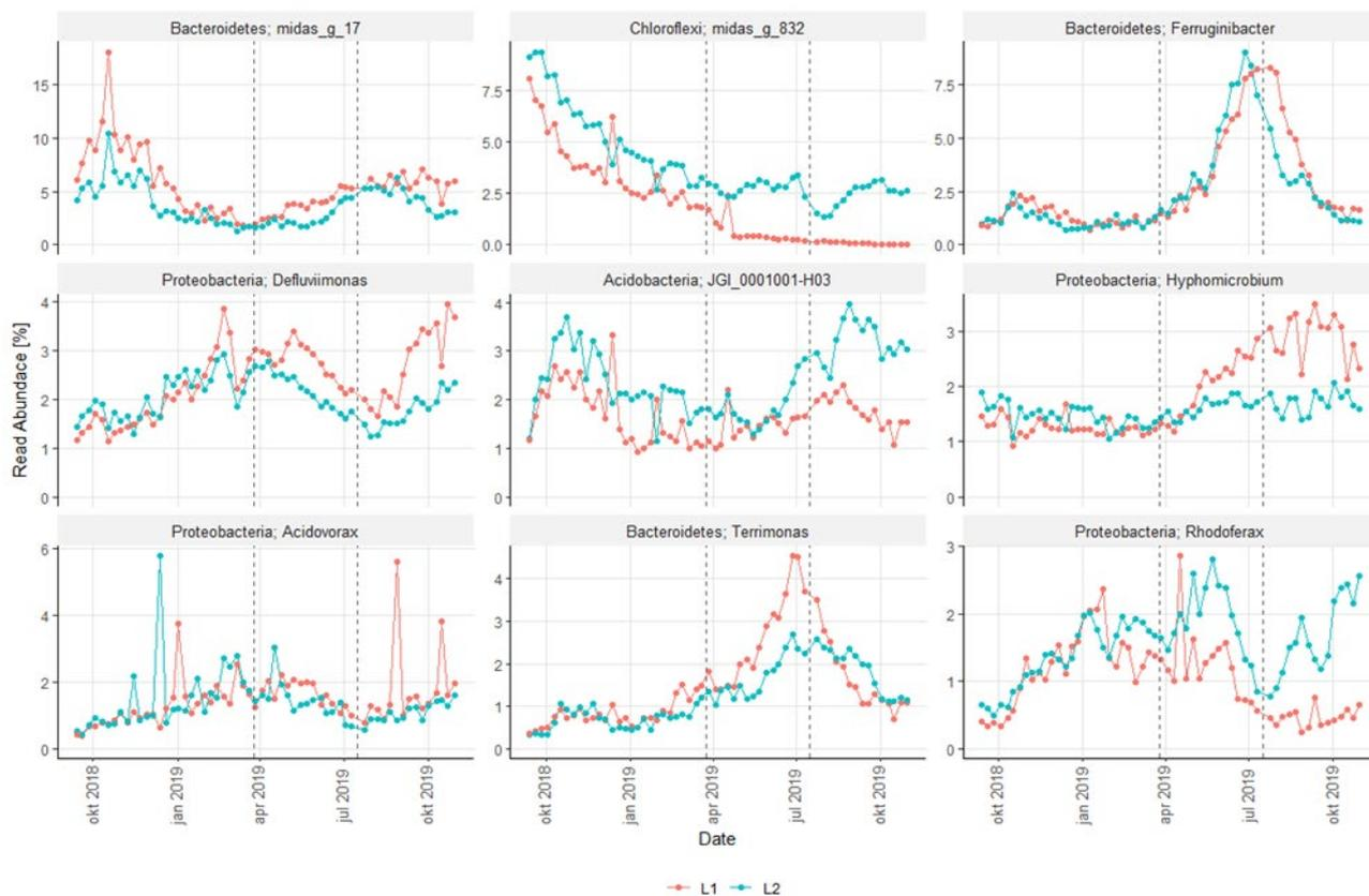
Figure 15 - Time series of other high abundant bacteria, with no/little known functions in activated sludge, in line 1 – experimental (red) and line 2 - control (blue). The dotted vertical lines represent the start of the two ozone conditions. Note the Y-axis varies in the figures.
