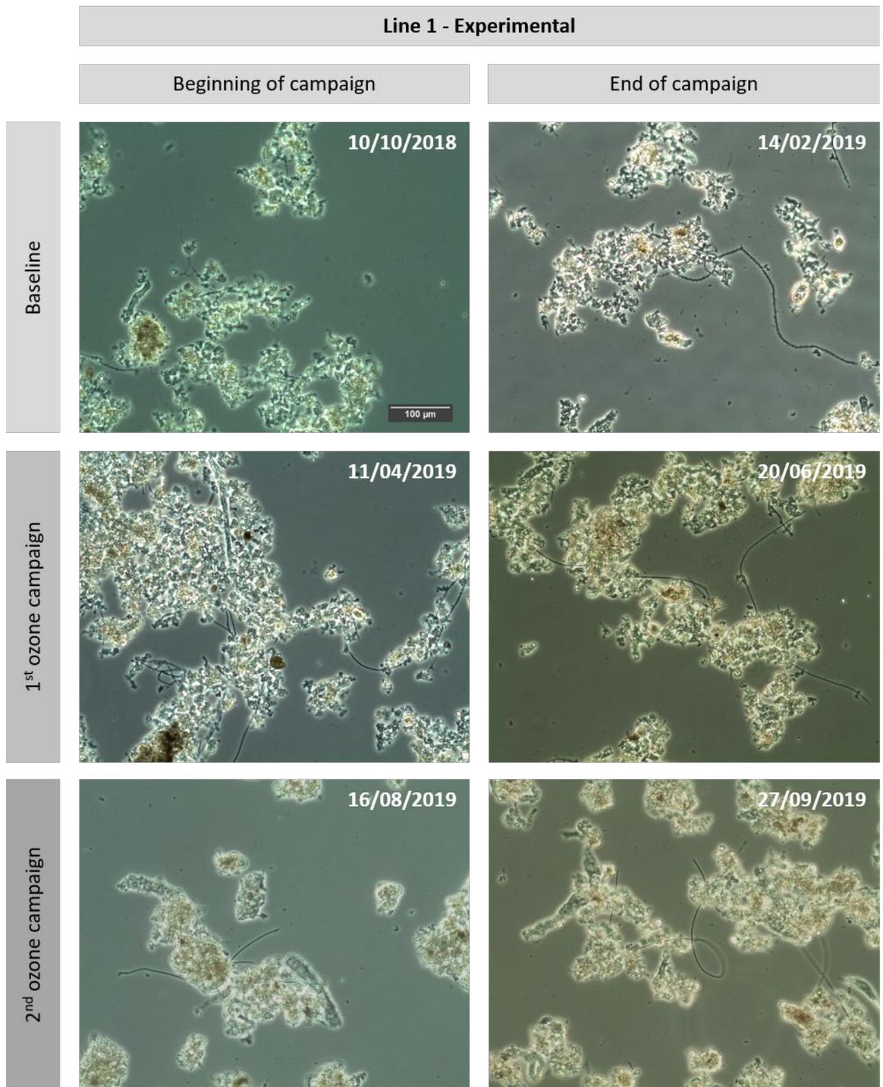
Figure 5 - Microscopic observation from Line1 - "Experimental". Development of floc structures during baseline campaign, ozonation condition and 2x ozonation condition.
