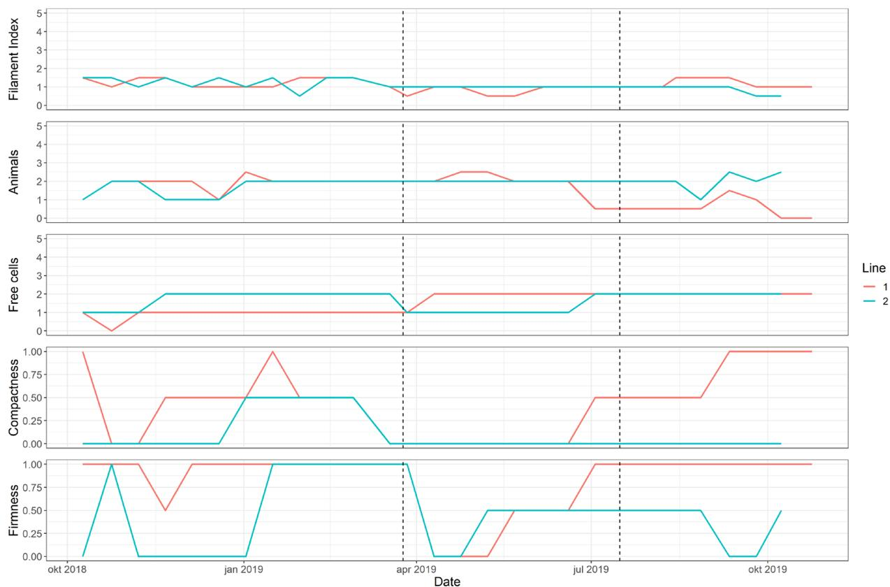
Figure 3 - Microscopic sludge investigation. Line 1 = experimental (red) and line 2 = control (blue). Dotted line represent start of ozonation condition 1 (3.98 mg/L ozone) and 2 (7.2 mg/L ozone). Filament Index, Animals and Free cells (scale from 0 = none, 5 = massive). Compactness (scale from 0 = diffuse to 1 = compact) and Firmness (scale from 0 = weak to 1 = firm).
