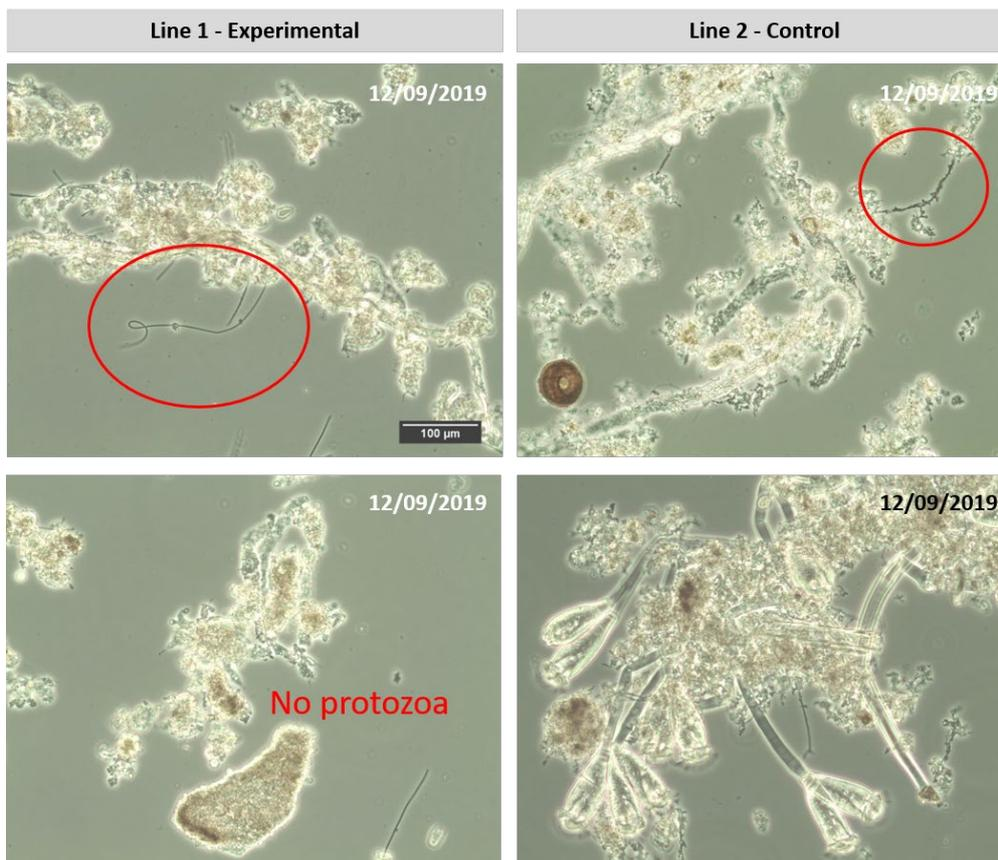
Figure 4 - Notable effects of second ozone condition. No attached growth on the filaments in line 1. No animals present in the experimental line 1, whereas the control line 2 had Vorticella, Arcella and Nematodes (not shown).
