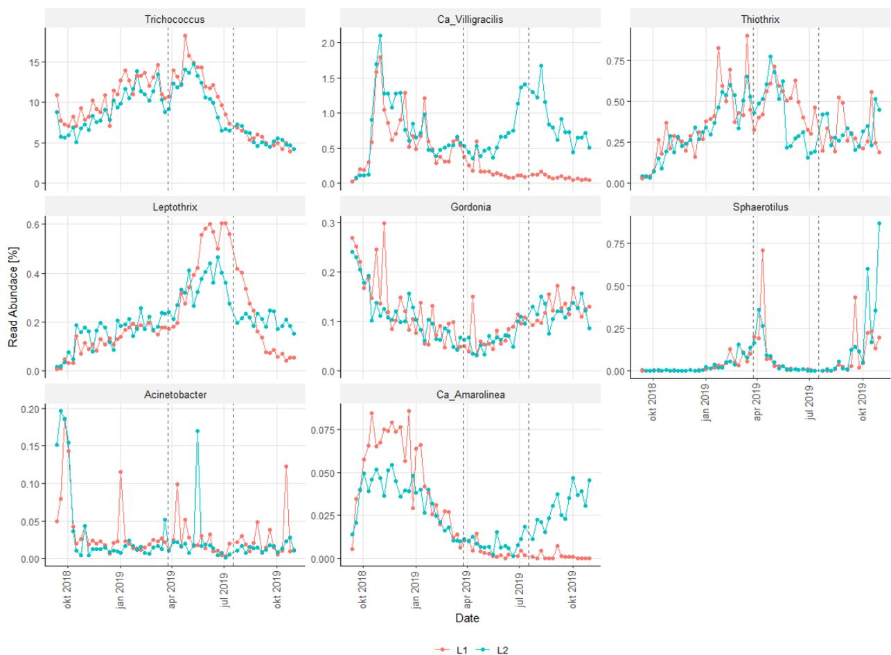
Figure 13 - Time series of known genera with filamentous morphology in line 1 – experimental (red) and line 2 - control (blue). The dotted vertical lines represent the start of the two ozone conditions. Note the Y-axis varies in the figures.
