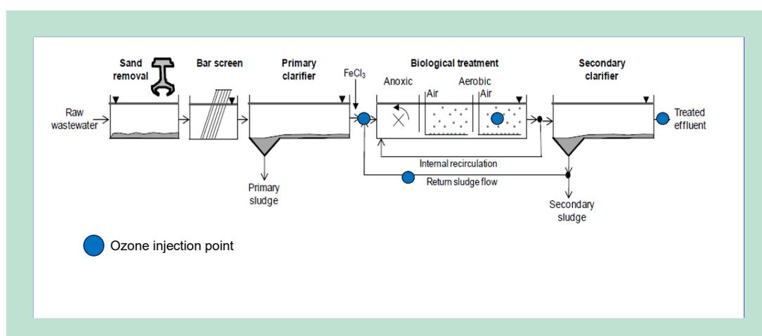
**FIGURE 7** Possible points of ozone injection to conventional wastewater treatment plant in multi points ozonation solution
