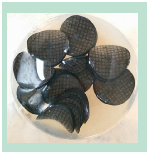
FIGURE 7. Z400 carriers with biofilm on the surface.
