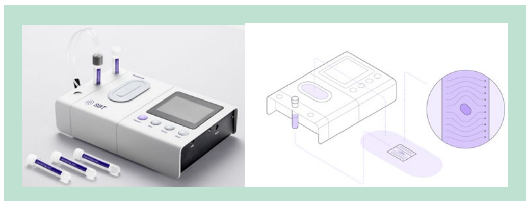
FIGURE 20. Impedance flow cytometry instrument BactoBox® (SBT Instruments) and measuring principle.
