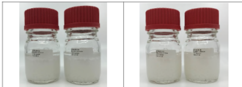
Figure 2: Picture of sample 970130-1 with product simulant (isooctane). The picture on the left is before the three-day migration and the picture on the right is after the migration. Note that no significant swelling is observed.
