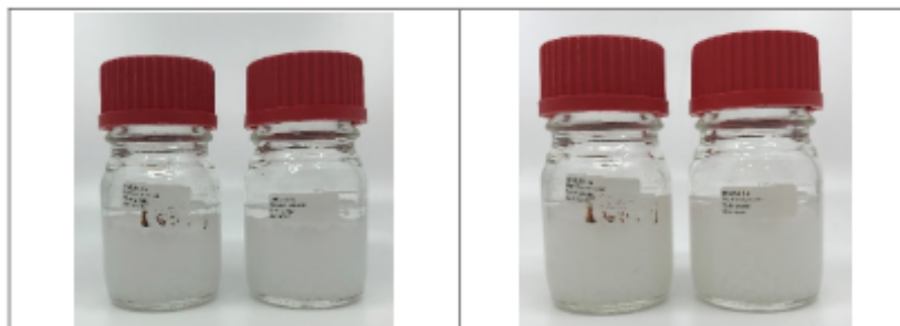
Figure 4: Picture of sample 970130-3 with product simulant (isooctane). The picture on the left is before the three-day migration and the picture on the right is after the migration. Note that no significant swelling is observed.
