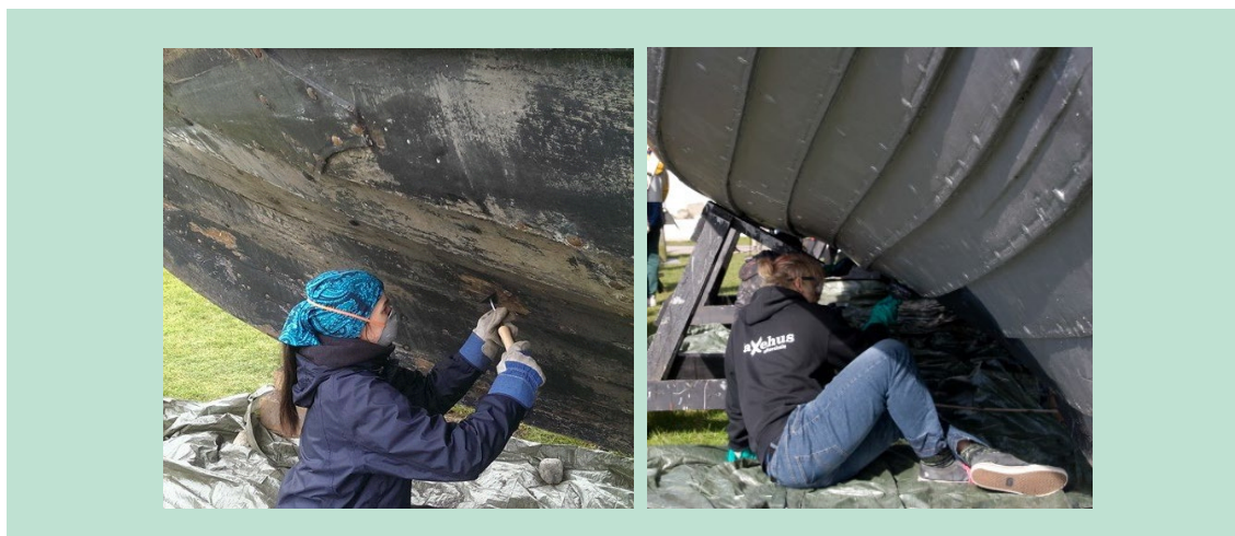
FIGURE 1: Removal of old AF paint (left) and repainting of the underwater boat hull (right).
