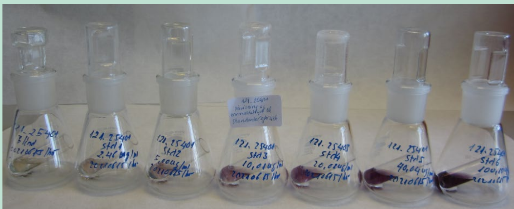
FIGURE 1. Prepared reference solutions including blank. From left: blank, 2.5 ppm formaldehyde, 5 ppm, 10 ppm, 20 ppm, 40 ppm, 100 ppm.
