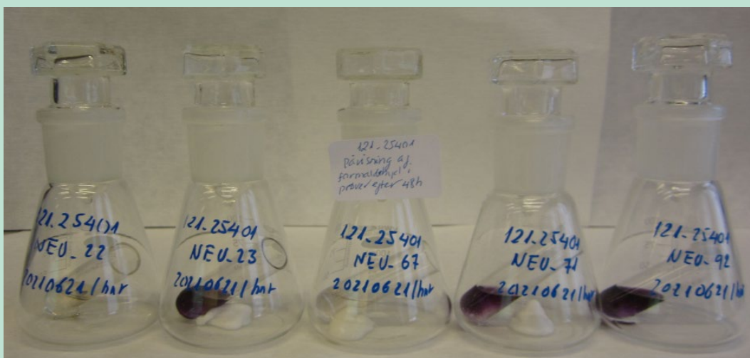
FIGURE 2. Examples of five of the analysed cosmetic products and the colour reactions developed. A precisely weighed quantity of the cosmetic product is placed in the bottom of the flask. Free formaldehyde degassing in the closed flask colours the liquid in the tube. The stronger the colour, the higher the concentration of free formaldehyde.
