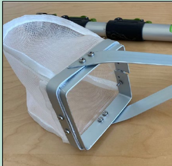
FIGURE 7. Scraper used to collect biological material associated with hard structures in the harbors.
