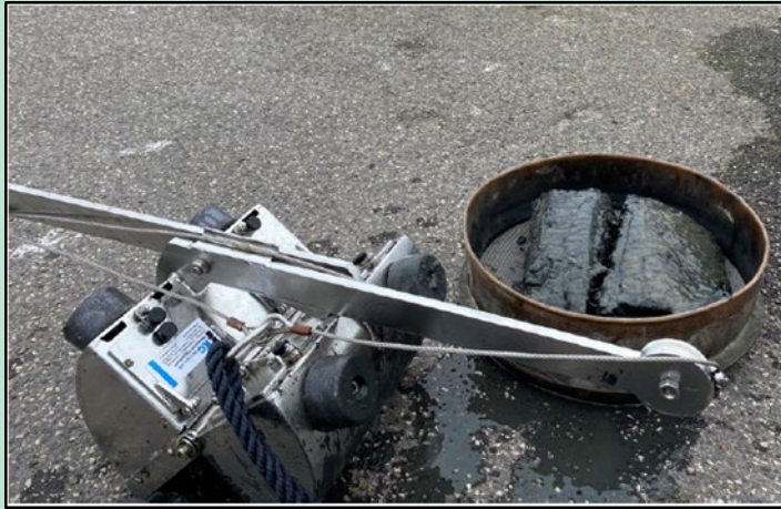
FIGURE 6. Hand-held Van Veen grab and 1 mm sieve used for soft bottom sampling in harbors.
