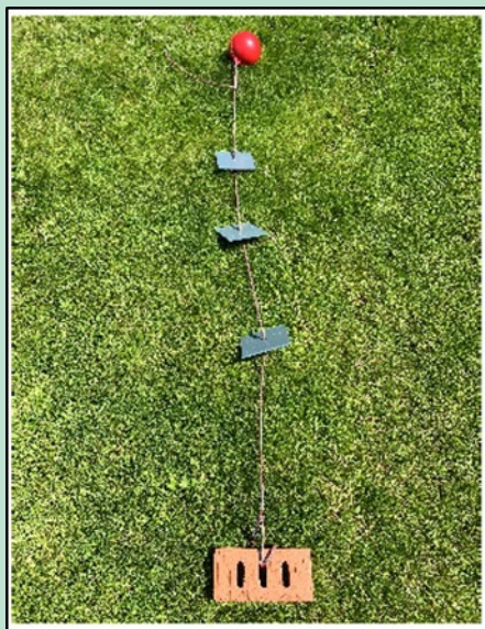
FIGURE 5. Settlement plates used for detection of NIS in three harbors.
