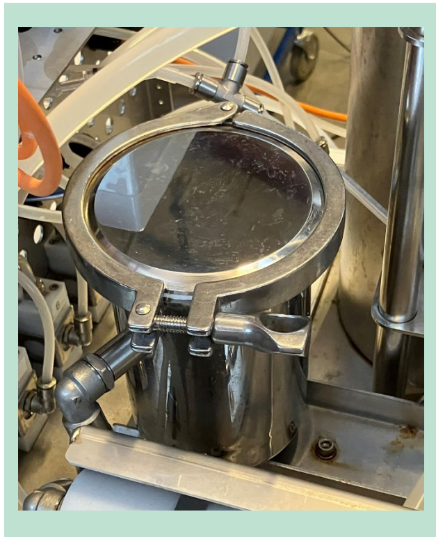
FIGURE 5. Sample container for the 10-50 µm size fraction, volume 1 L.
