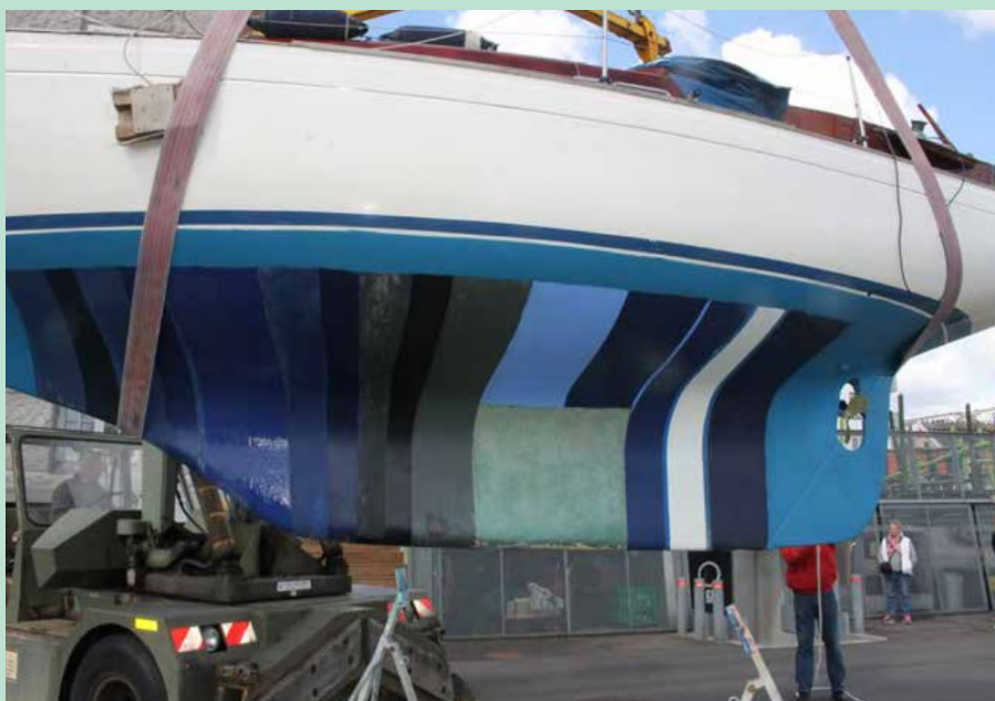
FIGURE 2-3 Test boat with application of different paints (from Rasmussen, 2021).
