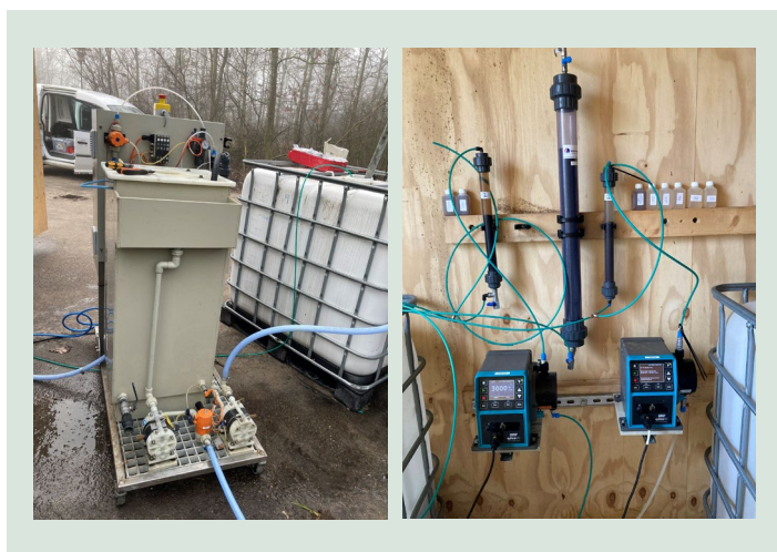
FIGURE 28. Left: Filtration system for treatment after coagulation/flocculation. Right: GAC (the column in the center) and resin columns.
