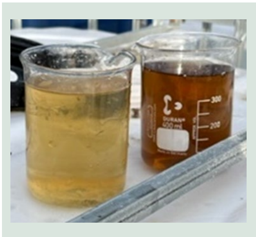
FIGURE 29. Leachate before (right) and after (left) ozonation treatment.
