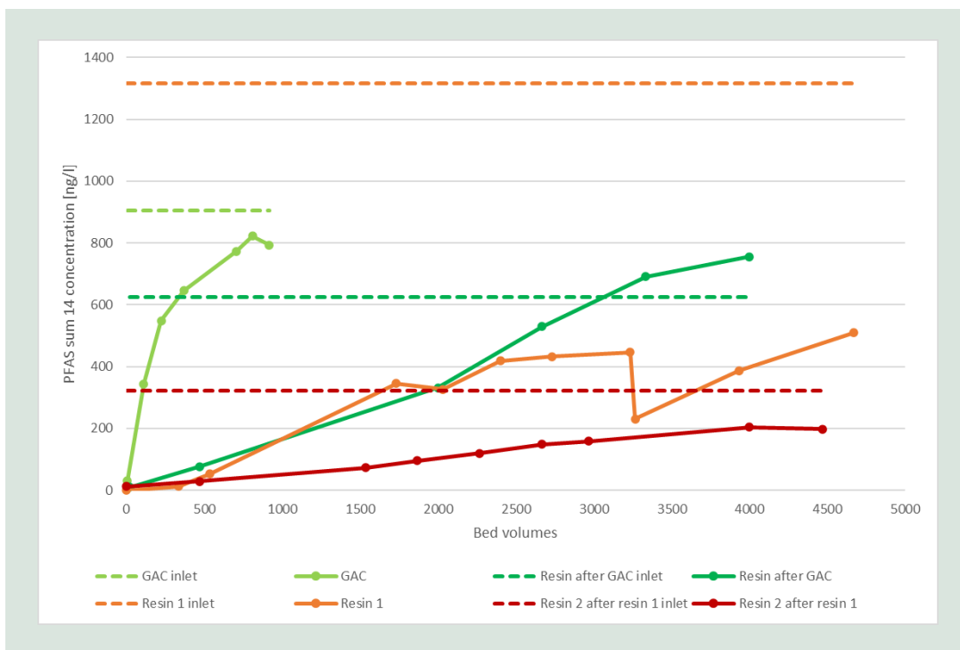
FIGURE 34. Monitored total PFAS sum 14 concentrations in outlet from different consecutive adsorption columns. The dotted lines represent inlet concentrations.
