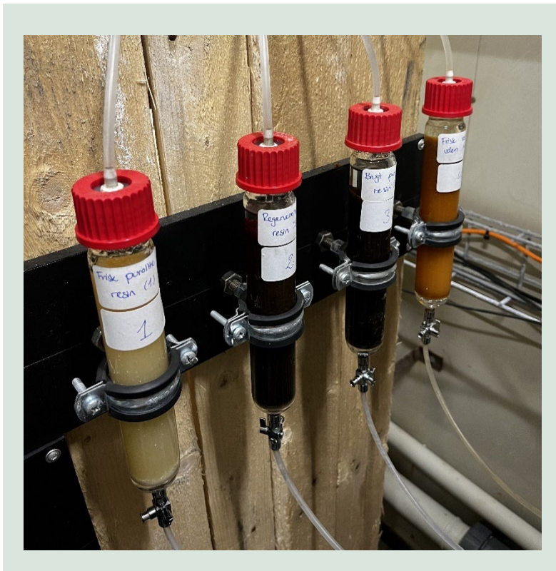
FIGURE 19. The four resin columns following one day of running. The column material in column four got increasingly darker as the experiment progressed.
