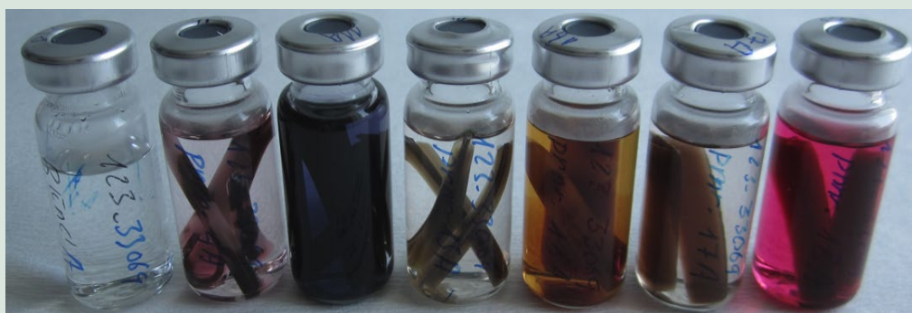
Figure 1. Colours of migration fluids immediately prior to GC-MS analysis, i.e., after 72 hours at 37 °C.
