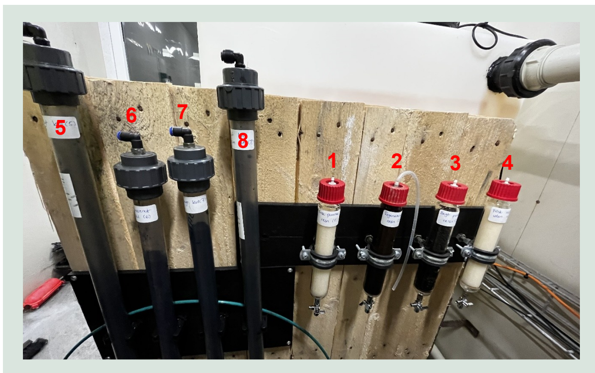
FIGURE 17. Columns one through eight during setup. Water is pumped in at the top and flows out through the bottom of each column.
