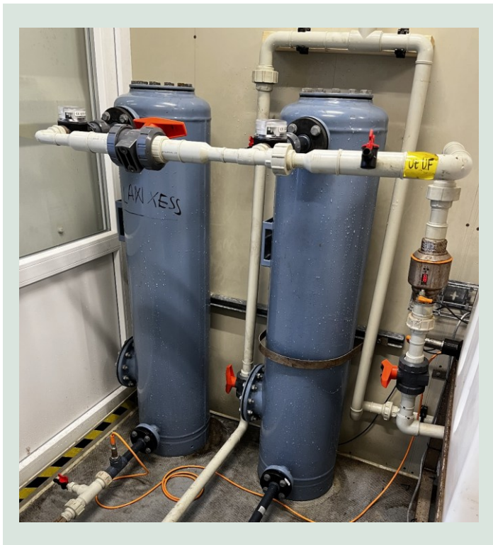
FIGURE 22. A parallel full-scale column set up containing ion-exchange resins. Experiments were conducted at Perpetuum landfill (Norway).
