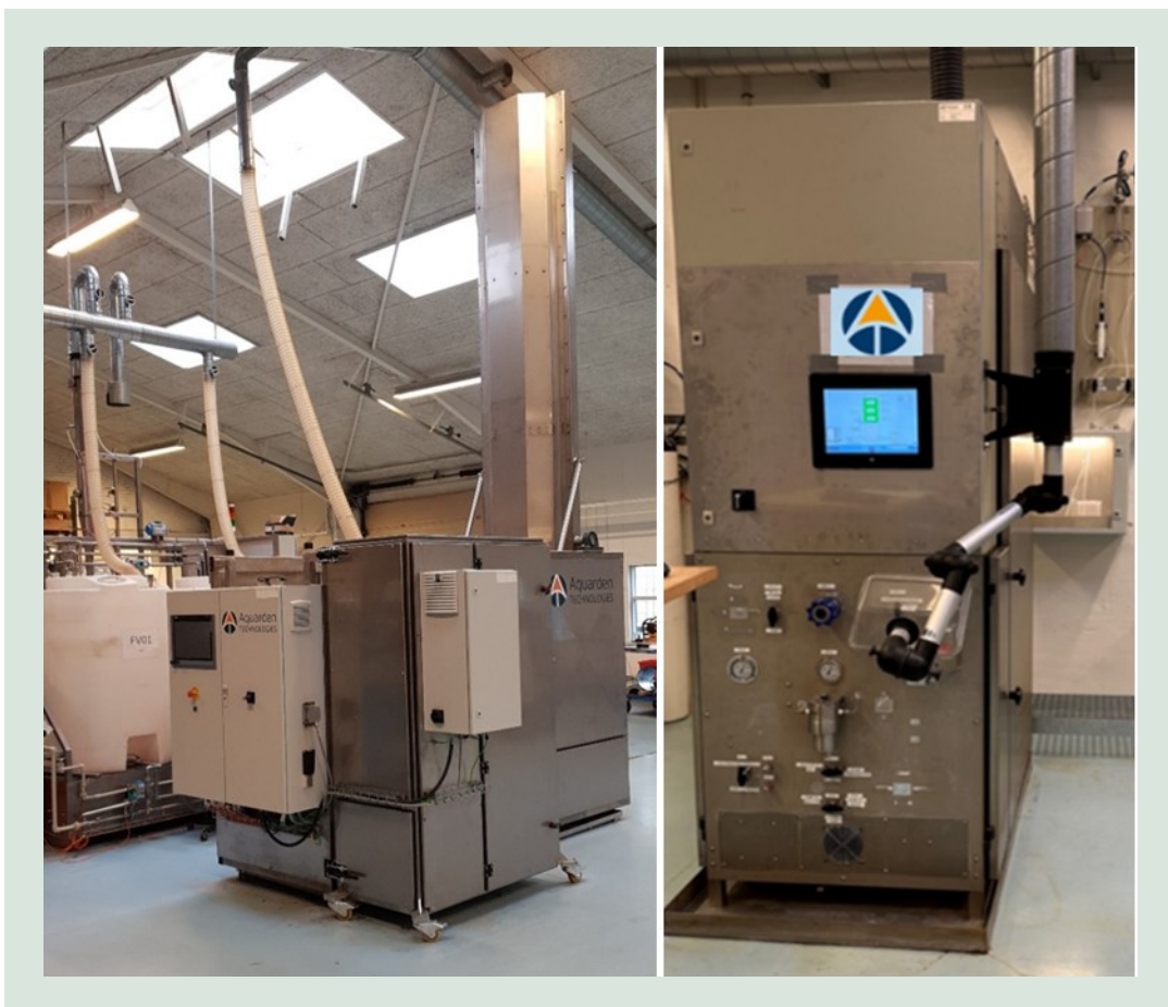
FIGURE 35. Aquarden’s SuperOx®, full-scale SCWO system (left) and laboratory-scale system (right).
