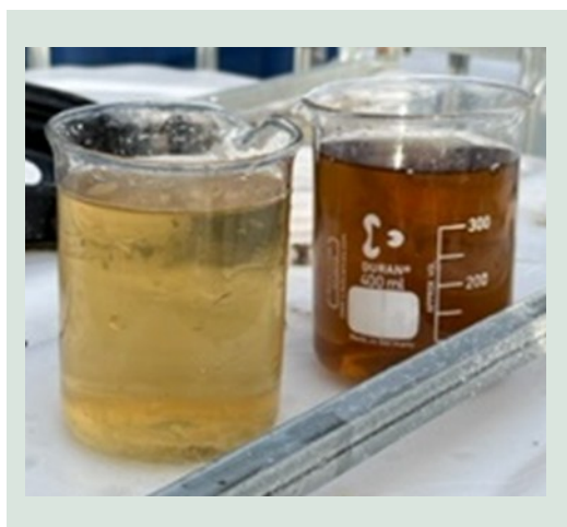
FIGURE 29. Leachate before (right) and after (left) ozonation treatment.
