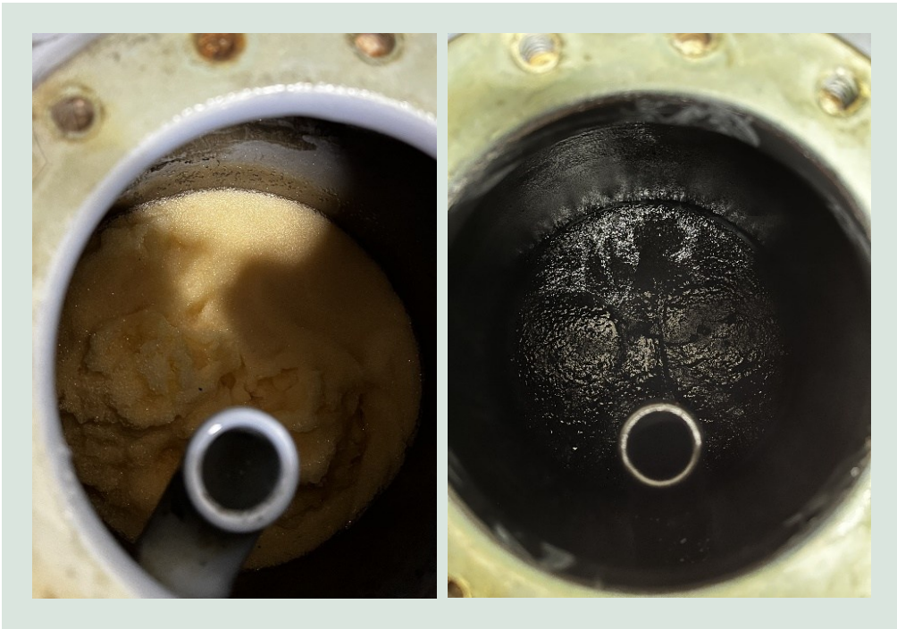
FIGURE 23. Resin before (left) and after (right) full-scale experiments at Perpetuum landfill (Norway).
