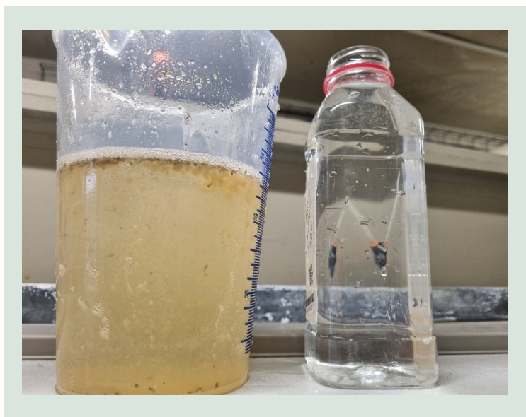
FIGURE 16. Raw leachate (left) and pretreated leachate (right).
