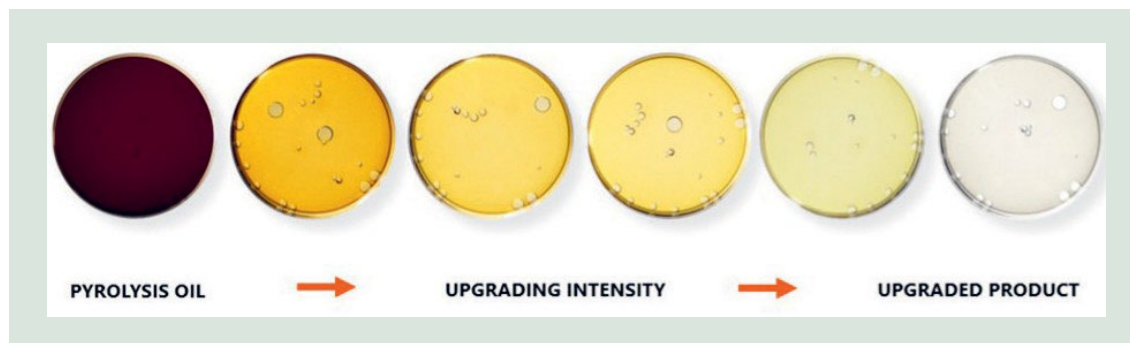
FIGURE 35. Illustration of the PureStep™ path from raw pyrolysis oil towards high-quality oil for plastic production.
