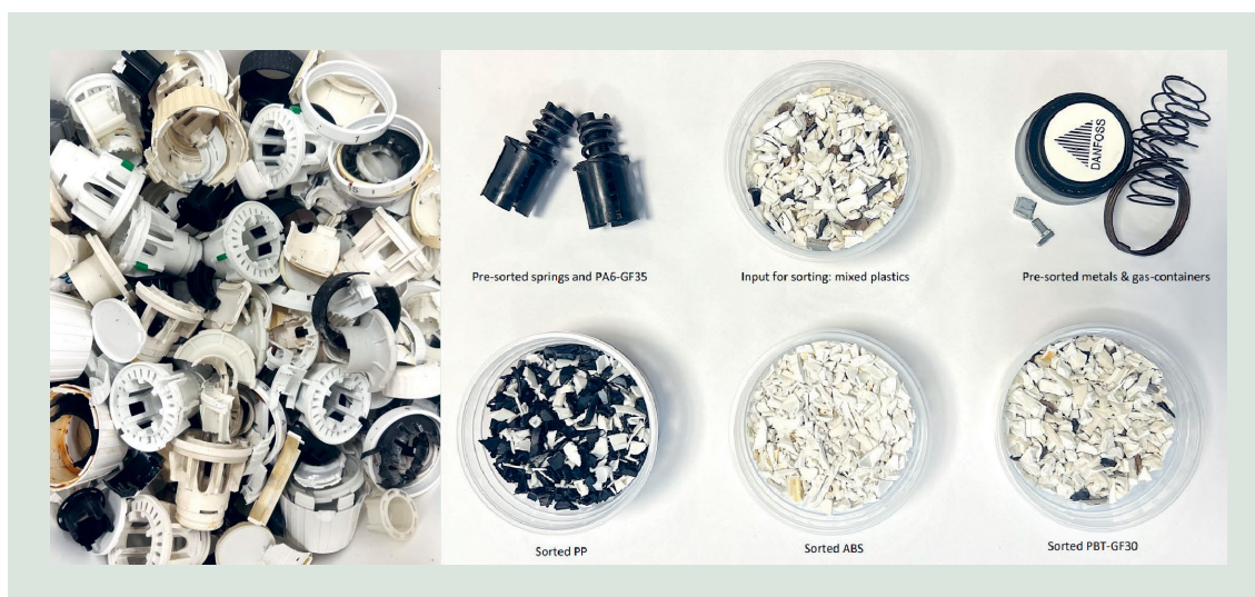
FIGURE 20. Plastics from end-of-life thermostats and resulting materials after test sorting at Trebo.
