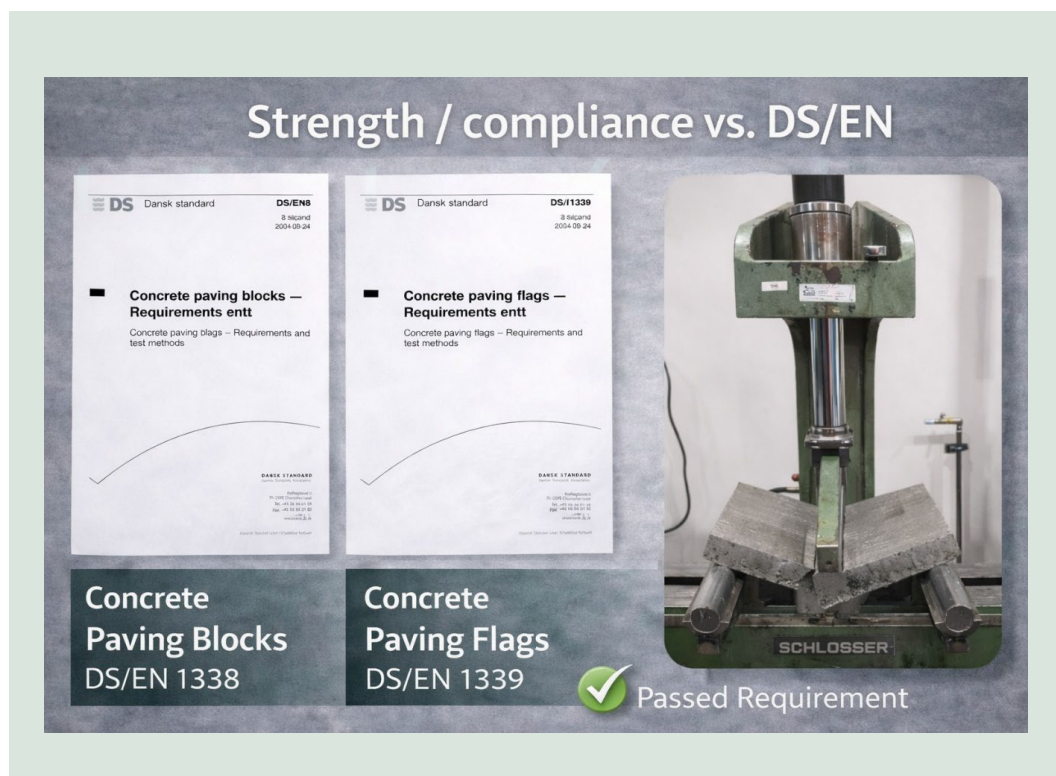
FIGURE 6. Mechanical performance and compliance with DS/EN 1338 and DS/EN 1339. Summary of mechanical validation confirming regulatory compliance under full-scale production.
