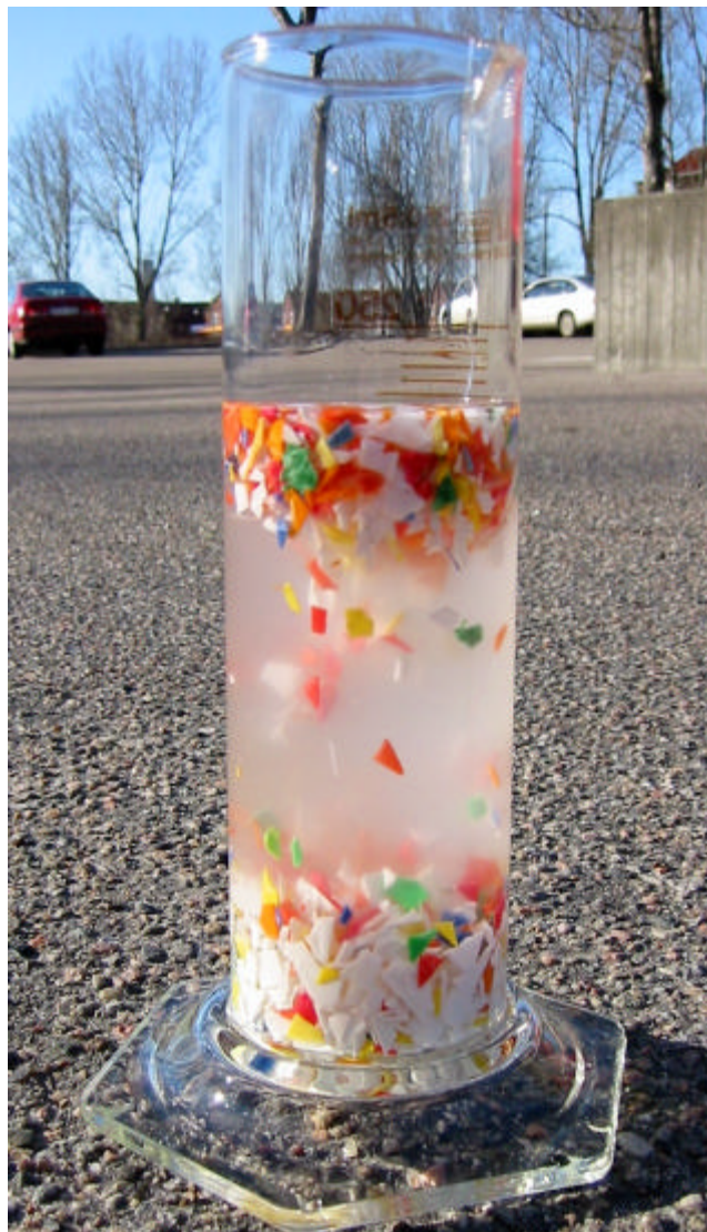
Figur 19 Separation i propanol/vand
