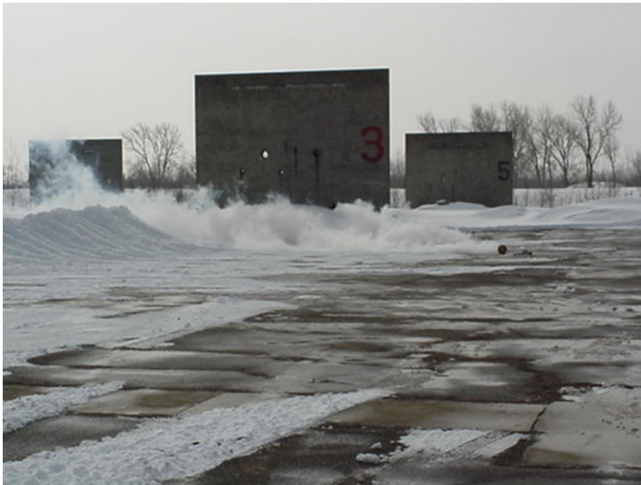
Figur 3.1 Udslip af ammoniak ved destruktion af en 15 l. cylinder. (Photo Dave Crosbie, Burnsville Fire Department and the Minneapolis Police Department Bomb Squad.) (15 liter udslip)
