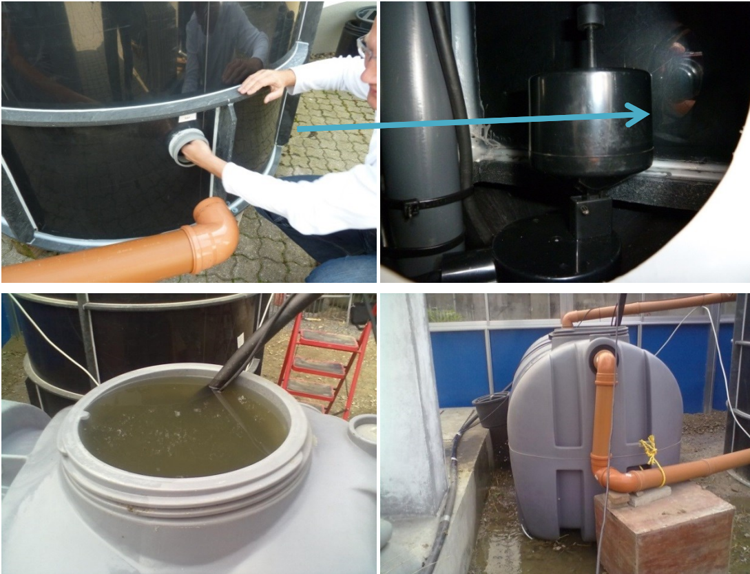
Figure 6.7 A defective floater device resulted in wastewater flooding at the test facility at several occasions in the beginning of the campaign. A new floater device and an overflow alarm system prevented further flooding incidents.
