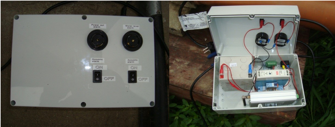
Figure 4.16 Alarm system installed in the Biokube system in Suzhou (June 2012)
