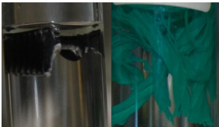
**Figure 4:** No observable changes after acidic treatment of polyolefins (PP left, HDPE right).
