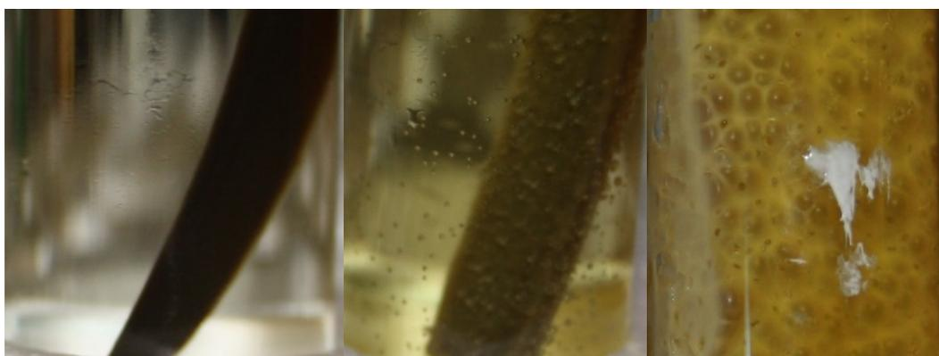
**Figure 1:** ABS bloating by acidic treatment after 5 h (left), 10 h (middle) and additional heating to 80°C (right).
