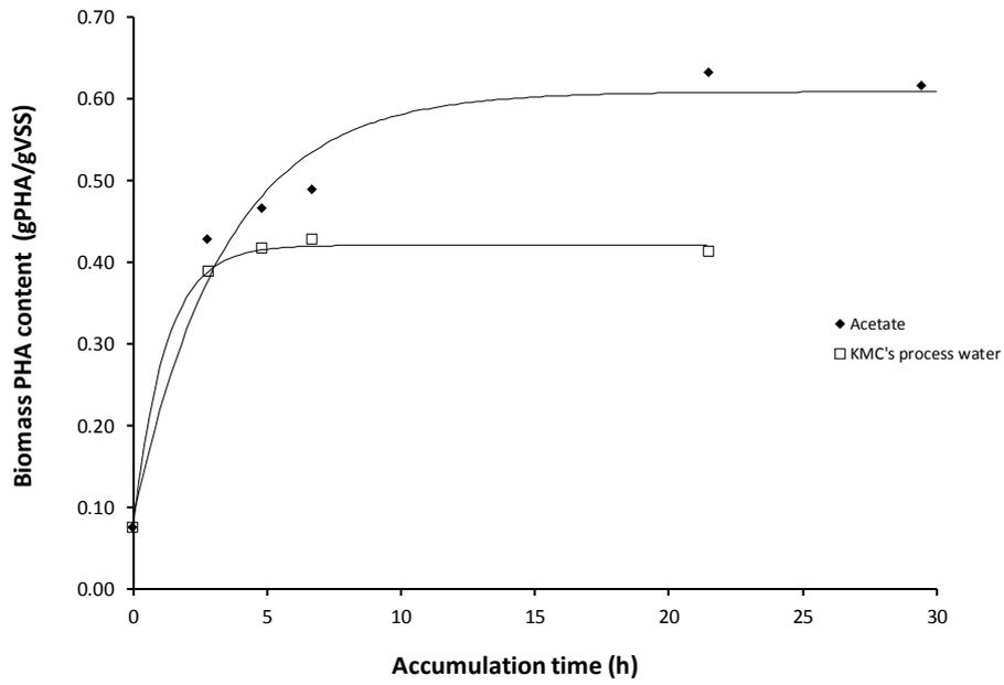
Fig. 14. Comparative lab-scale PHA accumulations with PE2 biomass (2015.05.20) using as feedstocks KMC process effluent and acetate
