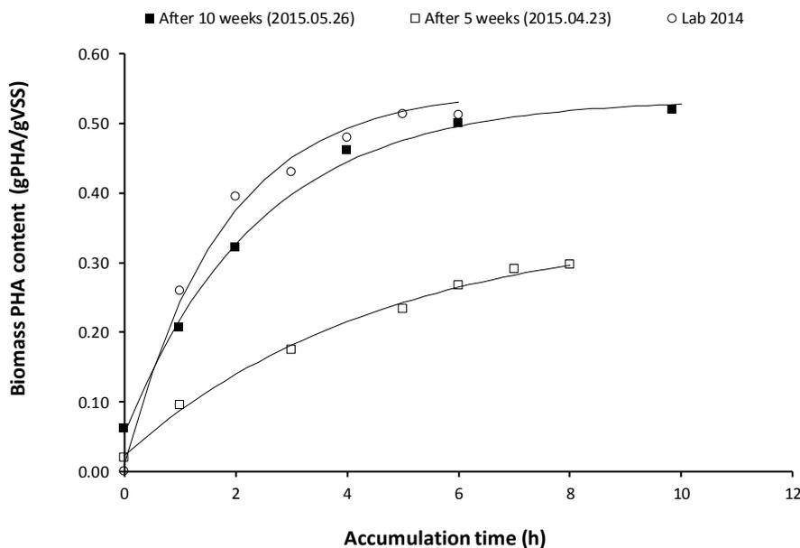
Fig. 12. PHA-accumulation response of biomass enriched with KMC process effluent upon addition of KMC process effluent as feedstock. Results for the pilot process biomass are shown after 5 and 10 weeks of operation, and from a lab-scale PHA accumulation in 2014.
