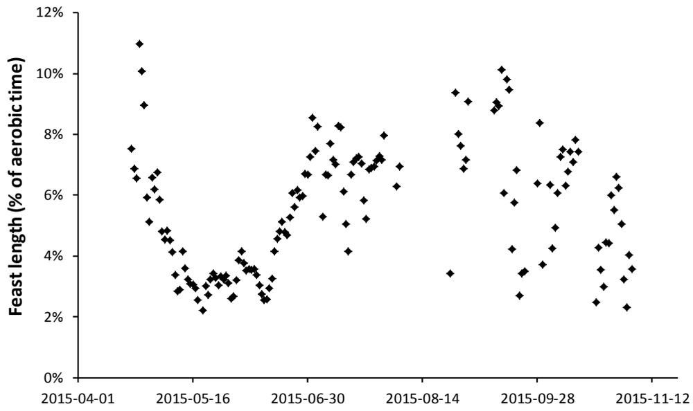
Fig. 11. Average cycle feast length as a percent of the aerobic (feast-famine) time per cycle (415 min) during the operating period
