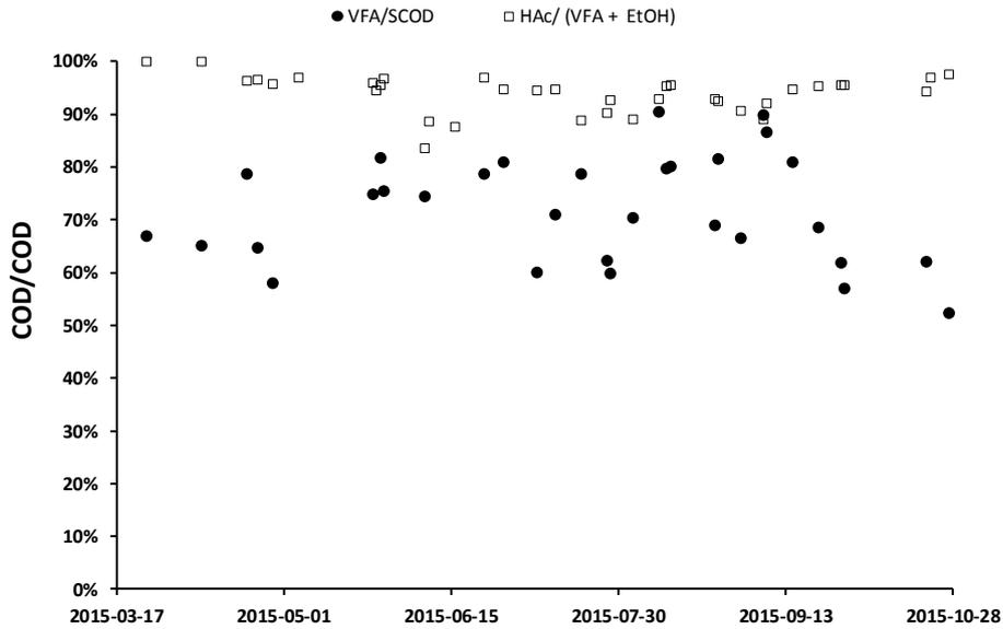
Fig. 5. COD quality in KMC process effluent as percent of acetic acid COD with respect to SCOD and with respect to the total VFA and ethanol COD as measured in the influent to the pilot process over time
