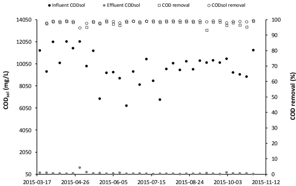
Fig. 6. Weekly average influent and effluent SCOD concentrations and COD removal efficiencies in the pilot process over time
