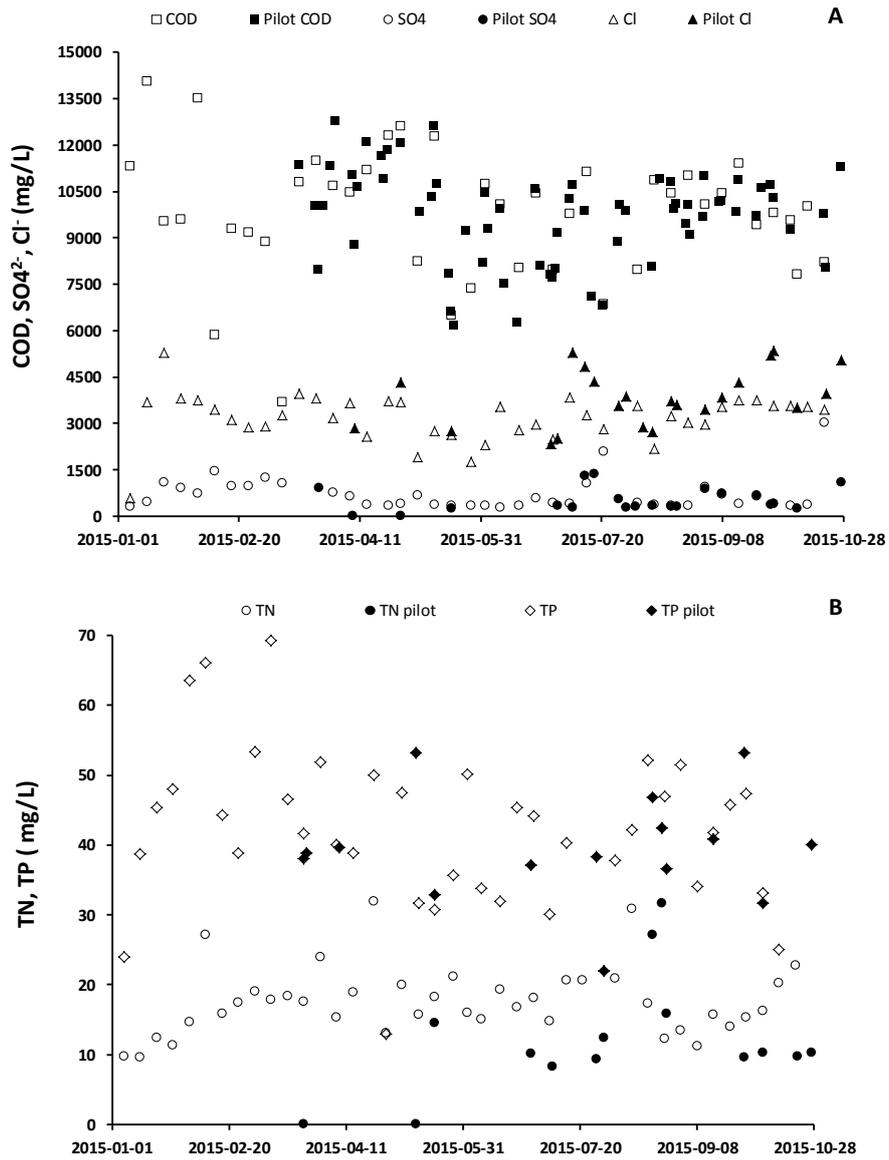
Fig. 4. COD, Cl<sup>-</sup> and SO<sub>4</sub><sup>2-</sup> (A) and total N and total P (B) concentrations in KMC process water effluent as measured in the influent to the pilot prototype and in the full-scale equalization tank during 2015
