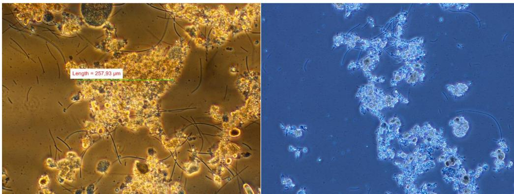
Fig. 9. Micrographs of typical activated sludge biomass with irregular, open floc structure and medium compactness (Samples from May 8 and 28, 2015).
