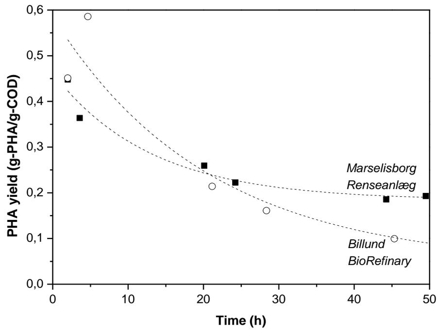
Figure 9. PHA yield during the accumulation tests with activated sludge from Marselisborg and BBR.
