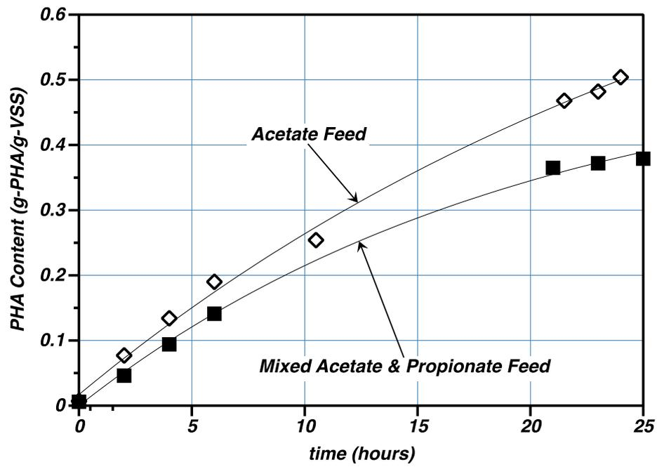
Figure 4. Summarized pilot scale PHA accumulation results with RWZI Bath biomass for PAP assessments using synthetic media for VFA feedstock.
