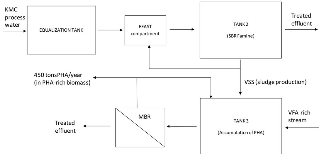
Figure E1. Envisioned potential operation of KMC treatment plant for the treatment of process water and production of a value-added PHAs with Cella™ Technologies.
