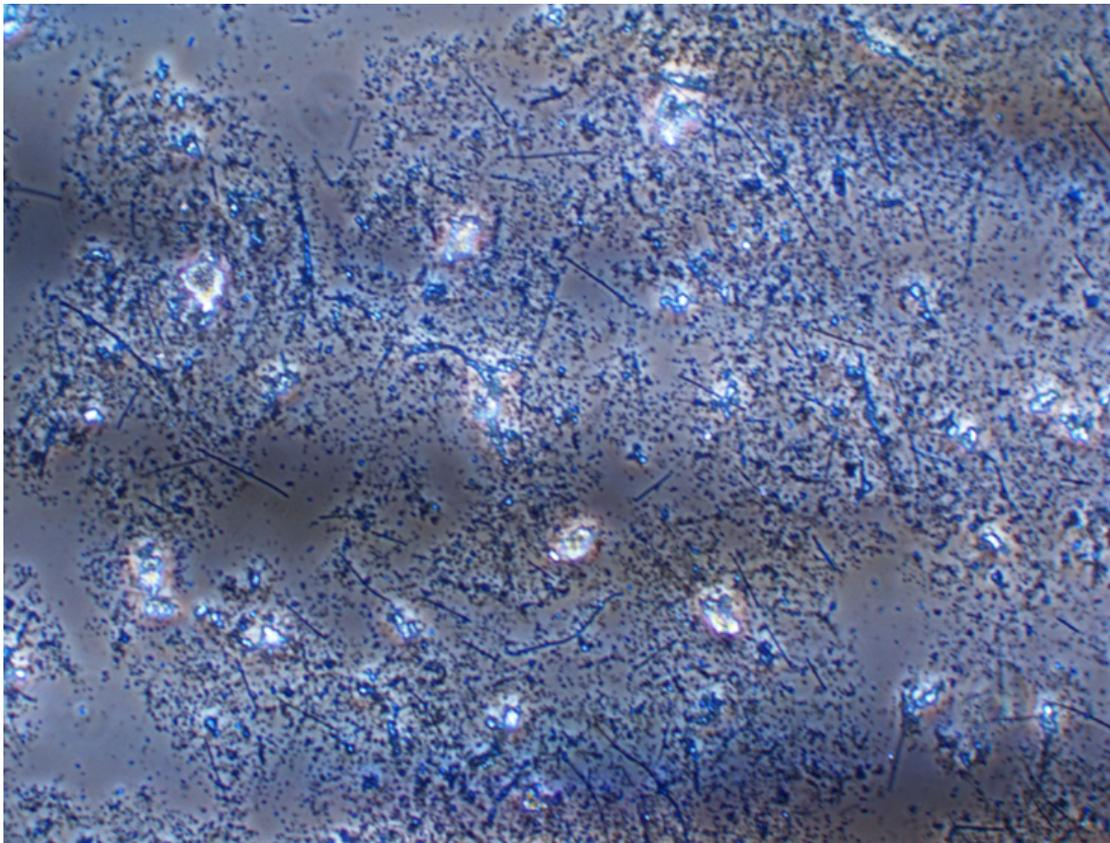
Figure 2. Picture (100x) of biomass harvested from Tank1 at KMC treatment plant (March 2015)
