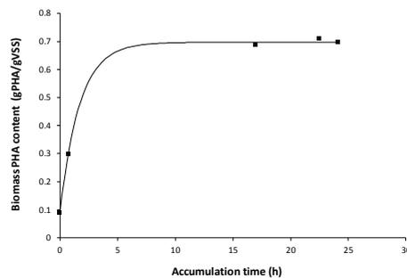
Fig.A1. PHA storage potential of KMC biomass from Cella™ pilot process operations (30°C, acetate)
