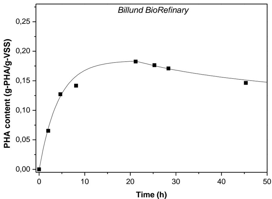
**Figure 8. Biomass PHA content during the accumulation test with activated sludge from Marselisborg Renseanlæg and Billund BioRefinery.**
