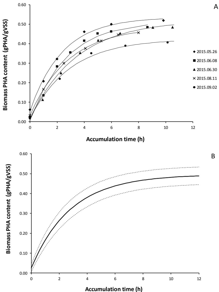
Fig. 13. PHA-accumulation response of pilot process biomass using as feedstock KMC process effluent at different points during the operating period (A) and as an average (solid line) with standard deviations (dotted lines) (B)
