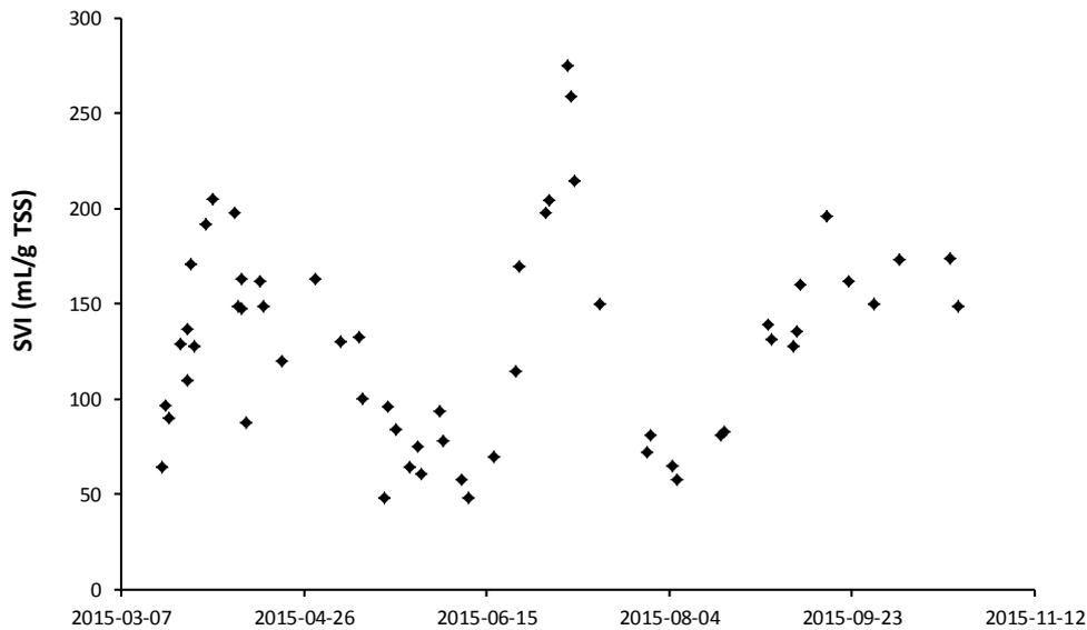
Fig. 7. SVI of the mixed liquor from the pilot process over time
