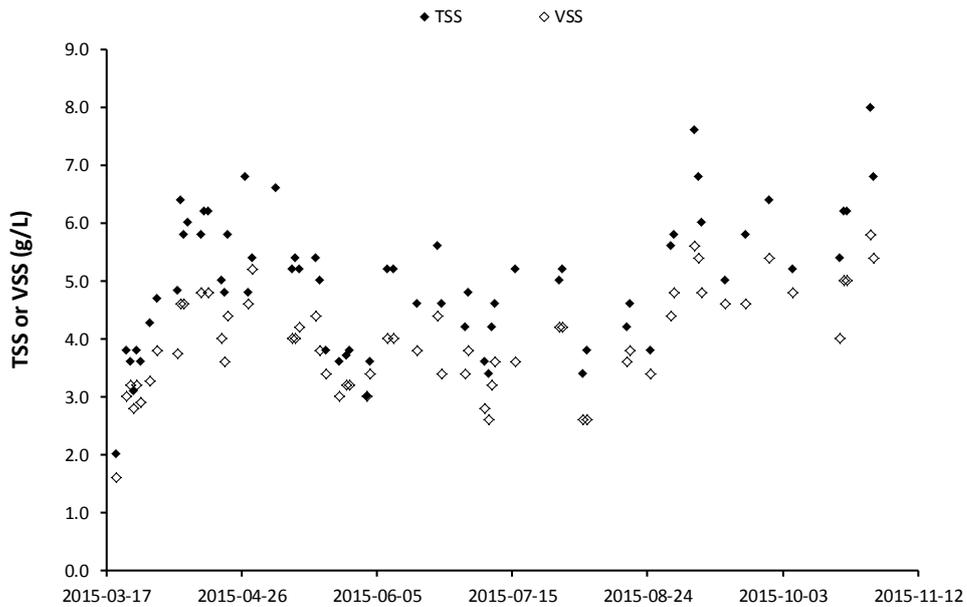
Fig. 8. Mixed liquor TSS and VSS levels in the pilot process over time
