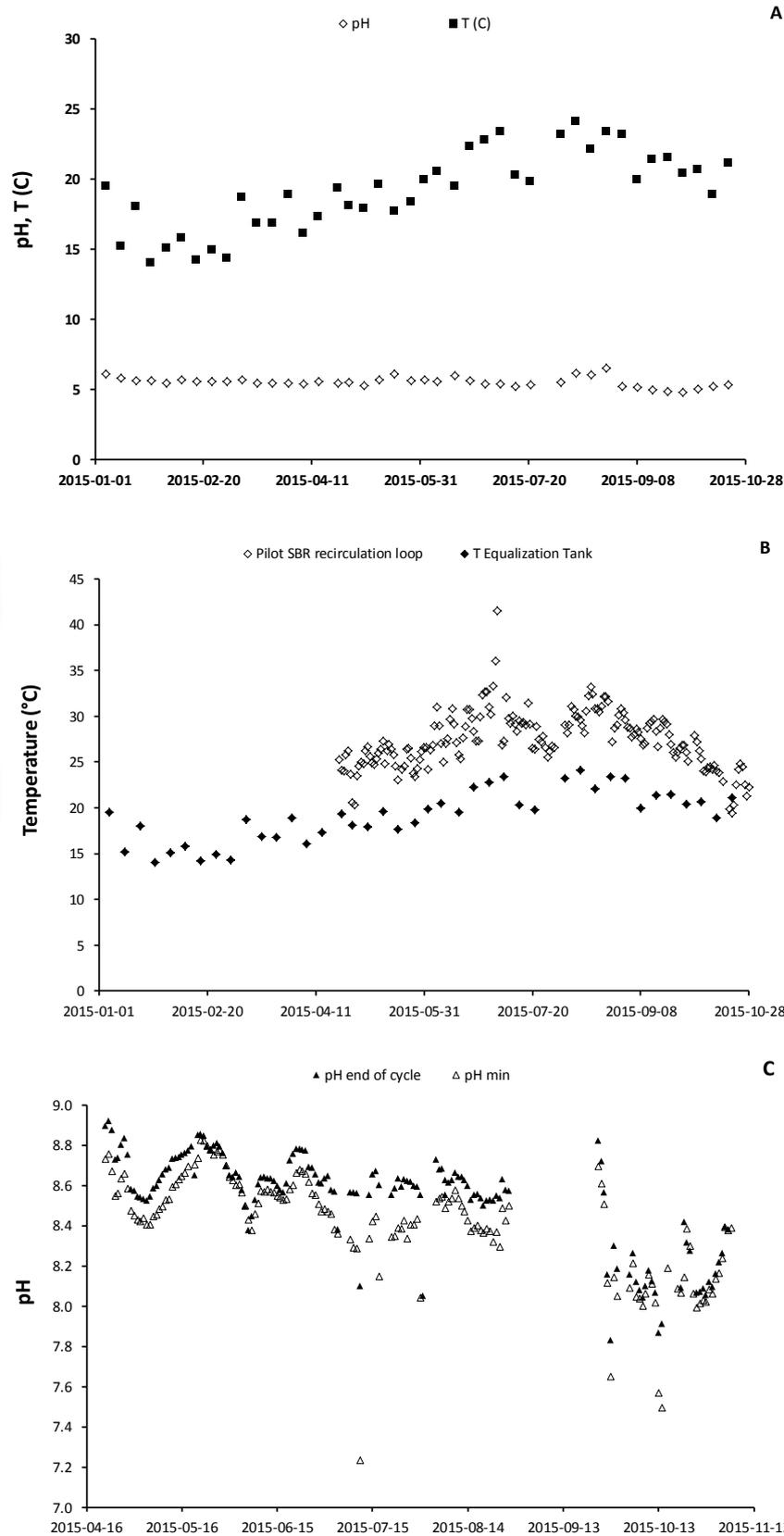
Fig. 3. Temperature and pH in KMC process effluent as measured in the equalization tank during 2015 (KMC's Drift Journal) (A) and in the mixed liquor of the pilot process measured in the recirculation loop (average of 3 cycles reported) (B, C)
