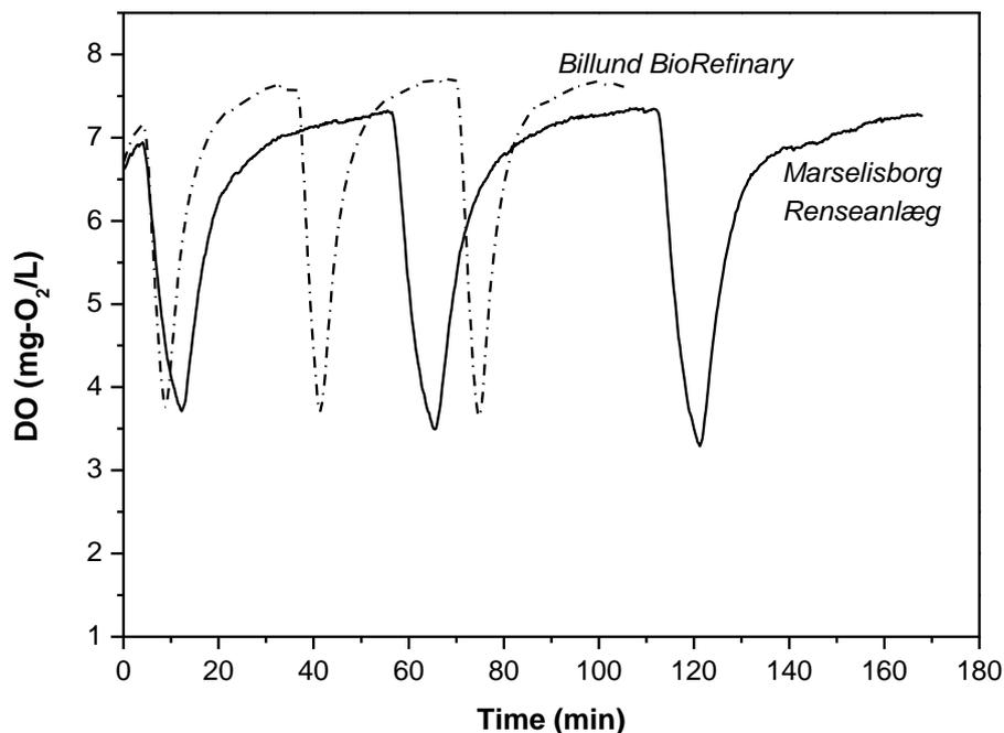
**Figure 6. DO concentrations under the pre-acclimation phase for the biomasses from Marselisborg Renseanlæg and Billund BioRefinery.**
