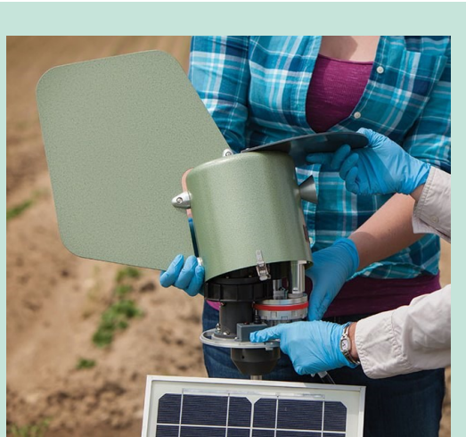
FIGUR 7 THE BURKARD MULTI-VIAL CYCLONE SAMPLER IN THE FIELD WITH THE COVER BEING REMOVED. PART OF THE SOLAR PANEL IS VISIBLE.
