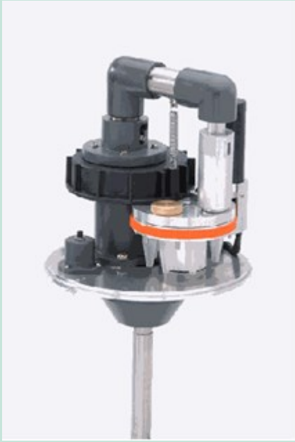
FIGUR 6 THE BURKARD MULTI-VIAL CYCLONE SAMPLER . THE VIALS (EPPENDORF TUBES) ARE VISIBLE.
