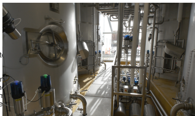
RO system for RO treatment of whey and its connection to the production system at Thise. (Copyright photo Thise Dairy)
