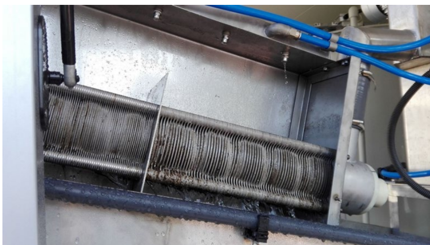
FIGURE 33. The screw press in operation. You see the moving plates.
