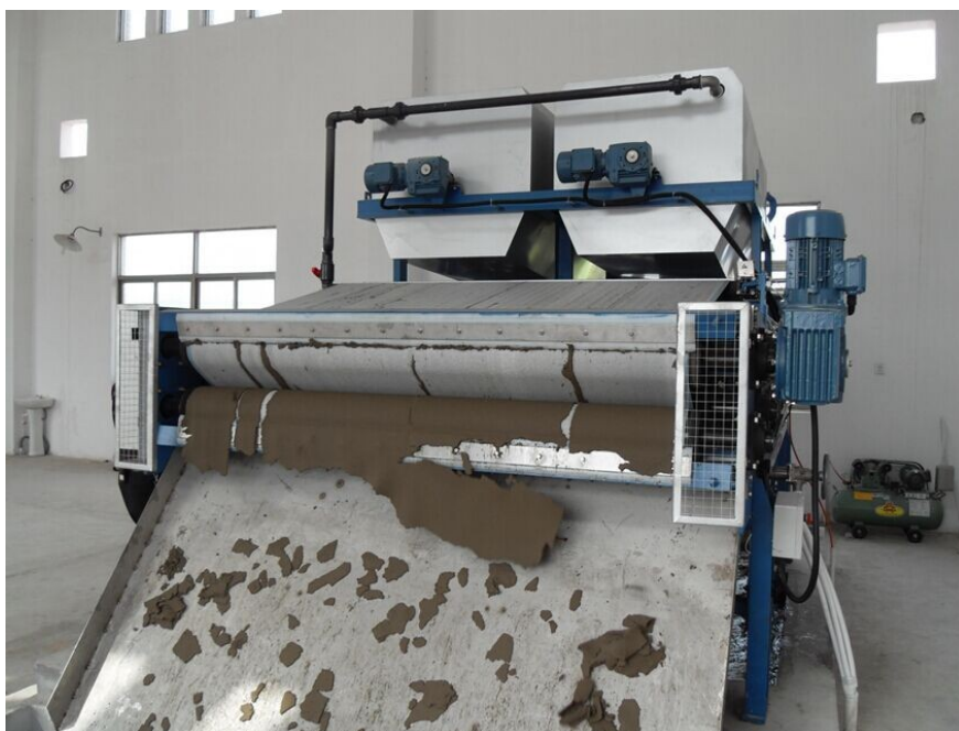
FIGURE 34. Sludge press in operation. You can see the sludge coming out of the system as dry matter with a dry matter content of over 18 %
