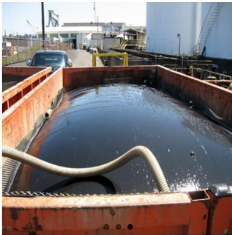
FIGURE 35. GeoTube in operation. The GeoTube bag is in the picture installed in a 20 foot garbage container for easy disposal.
