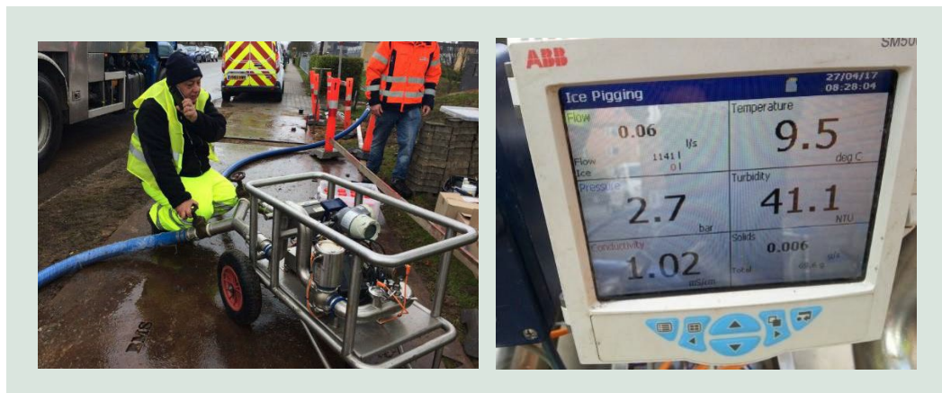
FIGUR 5. SUEZ Flow Analysis System (FAS-vogn) til feltmonitering.
