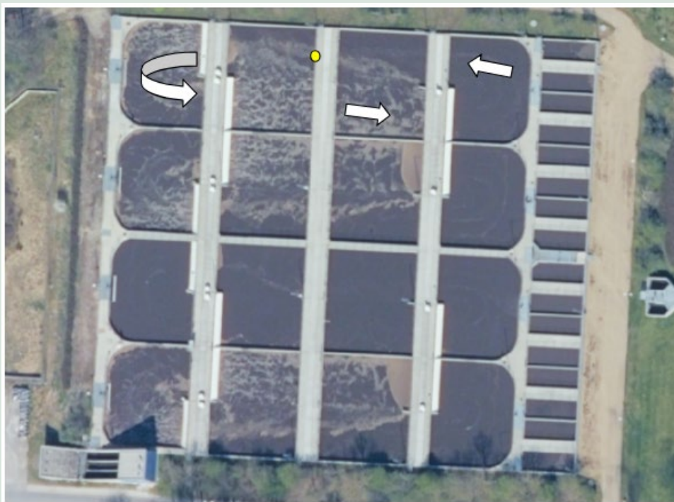
Figure B9. Case E: Næstved (NK – Spildevand A/S treatment facility) – a surface aerated system
