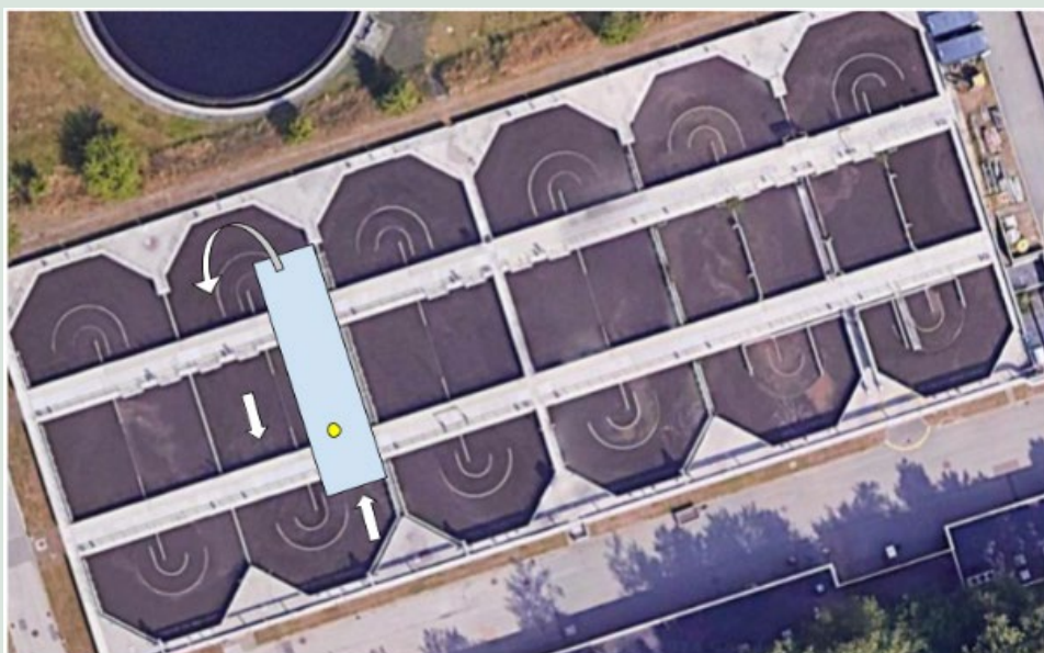
Figure B5. Case B: Mølleåværket treatment facility – a biodenitro system featuring bottom aeration
