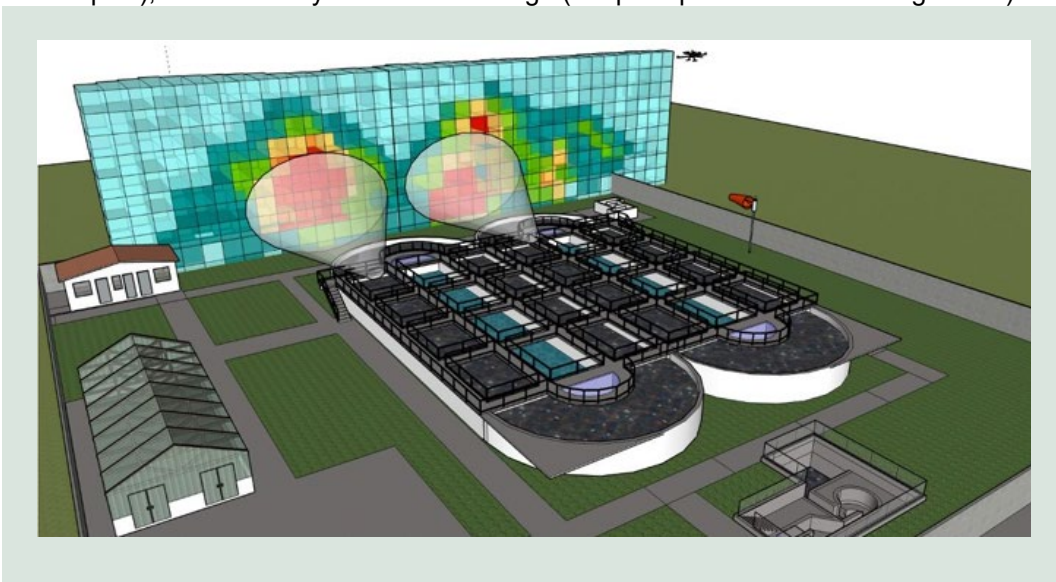
Figure B2: A schematic illustration shows the two-dimensional area in which the drone operates when mapping the nitrous oxide plume from a treatment plant. Adapted from Lallana, Arturo L. (2023), modified after Knudsen et al. (2022).
