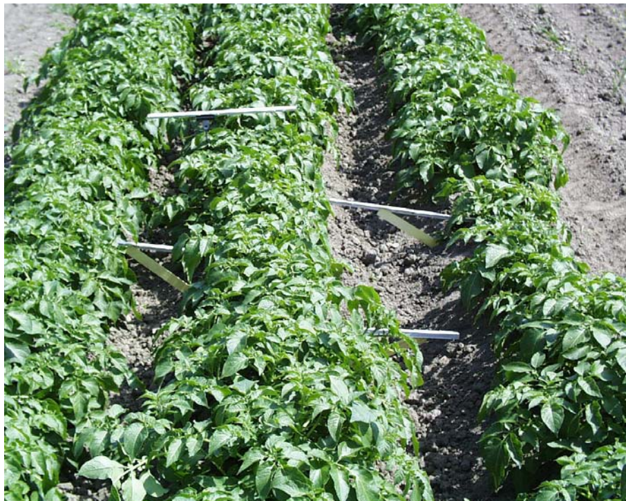
Figure 4. Placement of objects to catch spray at the soil surface and above the crop in potatoes when the plant cover exceeded approximately 50%.
