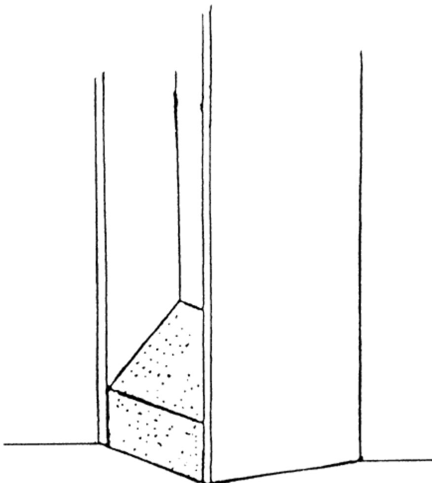
Cement filling provides easy cleaning and prevents pests
