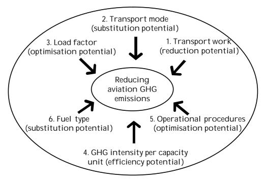
Figure 6:Examples of options for reducing greenhouse gas (GHG) emissions from commercial civil air transport. Source: [Nielsen 2001].
