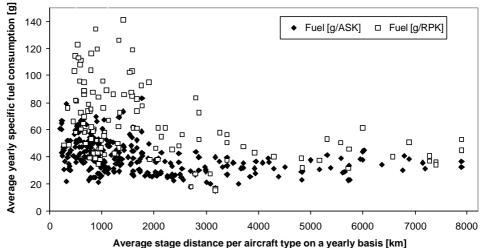
Figure 19: Specific fuel consumption per ASK and RPK versus stage distance for different types of aircraft. For an explanation of the data included see the explanations for Table 8 and Table 9. Data sources: [Premiair 2001] [All Nippon Airways 1999, 2000a and 2000b] [Lufthansa 1999 and 2000] [Lufthansa City Line 1999] [Swissair 1999] [SAS 1999b and 2000] [Sarames 1984] [Air Baltic 2001] [DOT 2001] [Norwegian Air Shuttle 2001] [AEA 1999]
