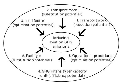
Figure 1:Examples of options for reducing greenhouse gas (GHG) emissions from commercial civil air transport. Source: [Nielsen 2001].
