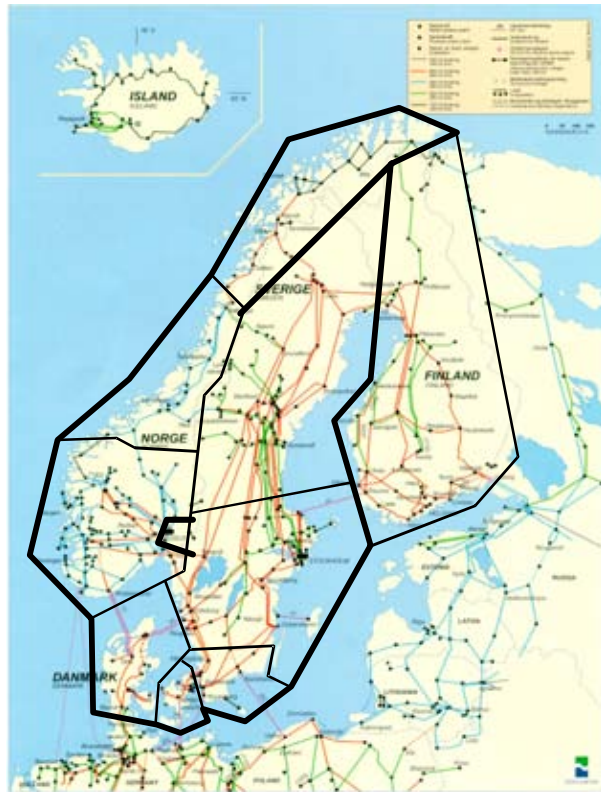
Figure 31: The 10 transmission areas, which the Nordic system consists of in the model.
