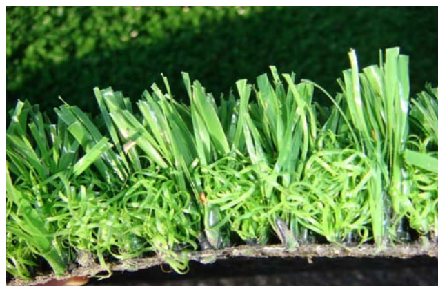
Figure 1.3 PE grass with polyamide support fibres
