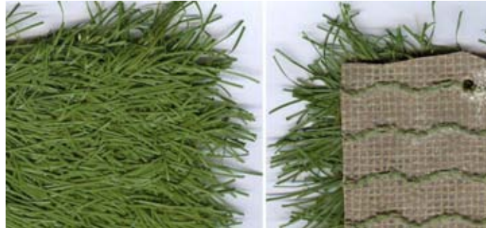
Figure 1.2 Mesh for artificial turf, front and back
