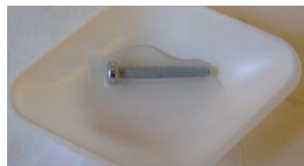
Chromium(VI)-free screw. No colour reaction is seen in a test solution or diluted test solution.
