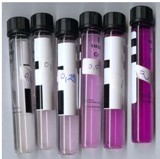
Figure 3 Colour scale - liquids for calibration: Concentrations in ppm from left: 0.05/0.1/0.2/0.5/1/2.
