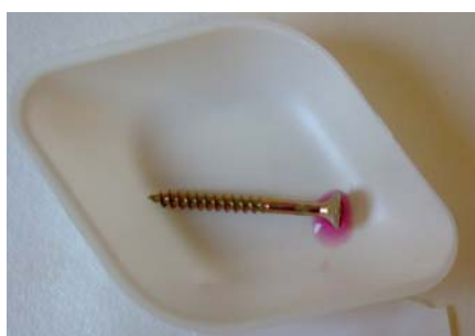
Yellow chromated screw with test solution. The characteristic reddish purple colour indicates the presence of chromium(VI).
