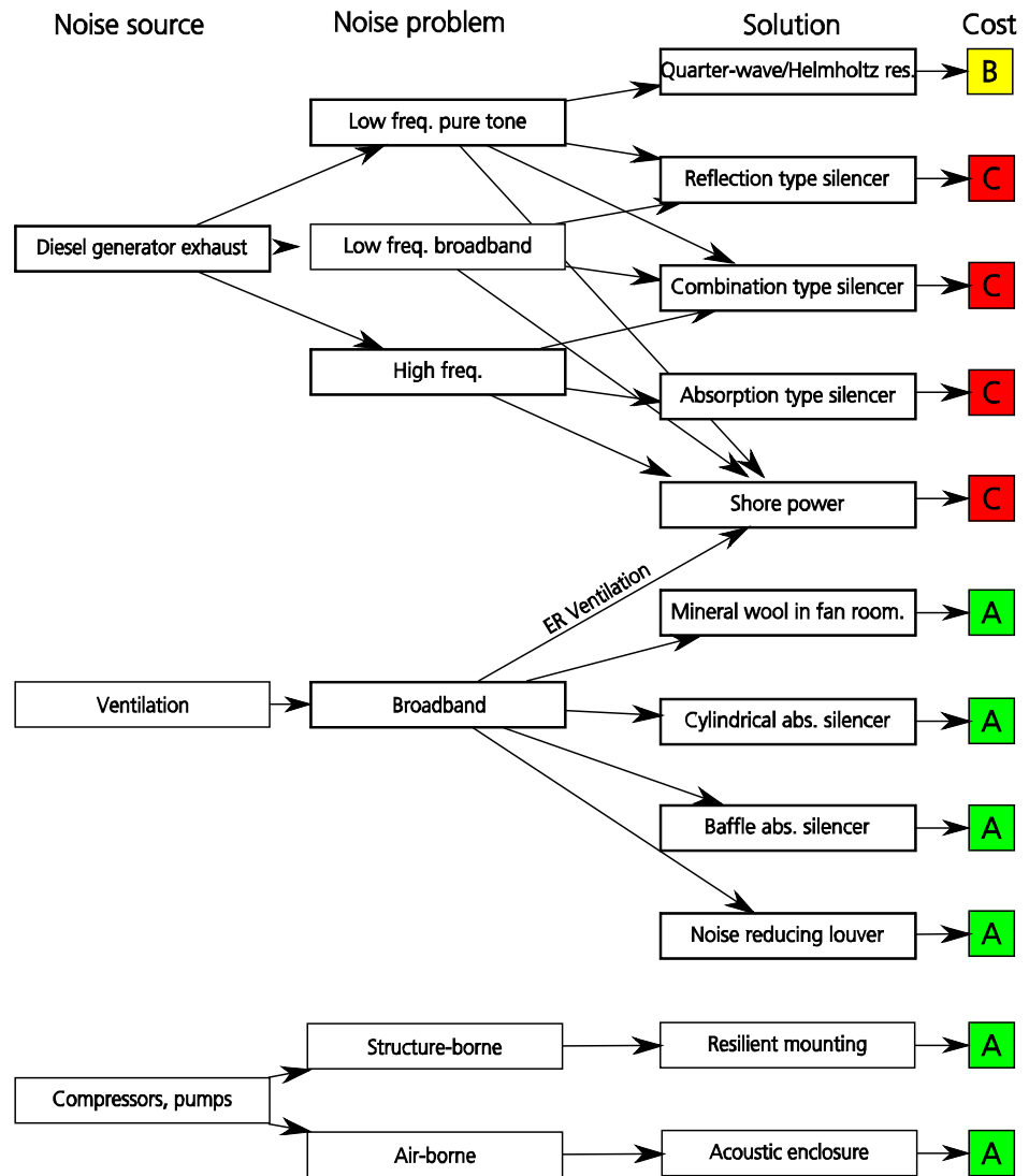
FIGURE 12 DIAGRAM OF DIFFERENT SOLUTIONS TO DIFFERENT EXTERNAL NOISE PROBLEMS AND THE APPROXIMATED COST OF THE SOLUTIONS. RED COLOUR AND THE LETTER C INDICATES ESTIMATED HIGHEST COST, YELLOW COLOUR AND THE LETTER B INDICATES ESTIMATED LESS COST AND GREEN COLOUR AND THE LETTER A INDICATES ESTIMATED LEAST COST.
