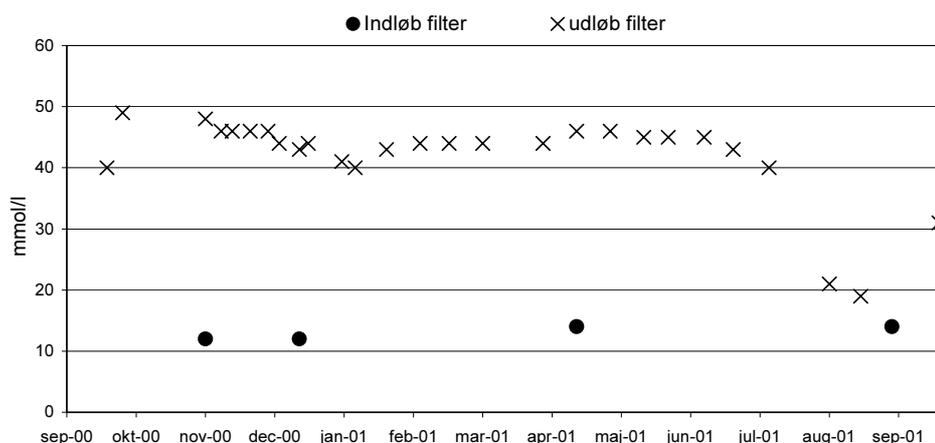
FIGUR 22: ALKALINITET I FILTERETS IND- OG UDLØB.
