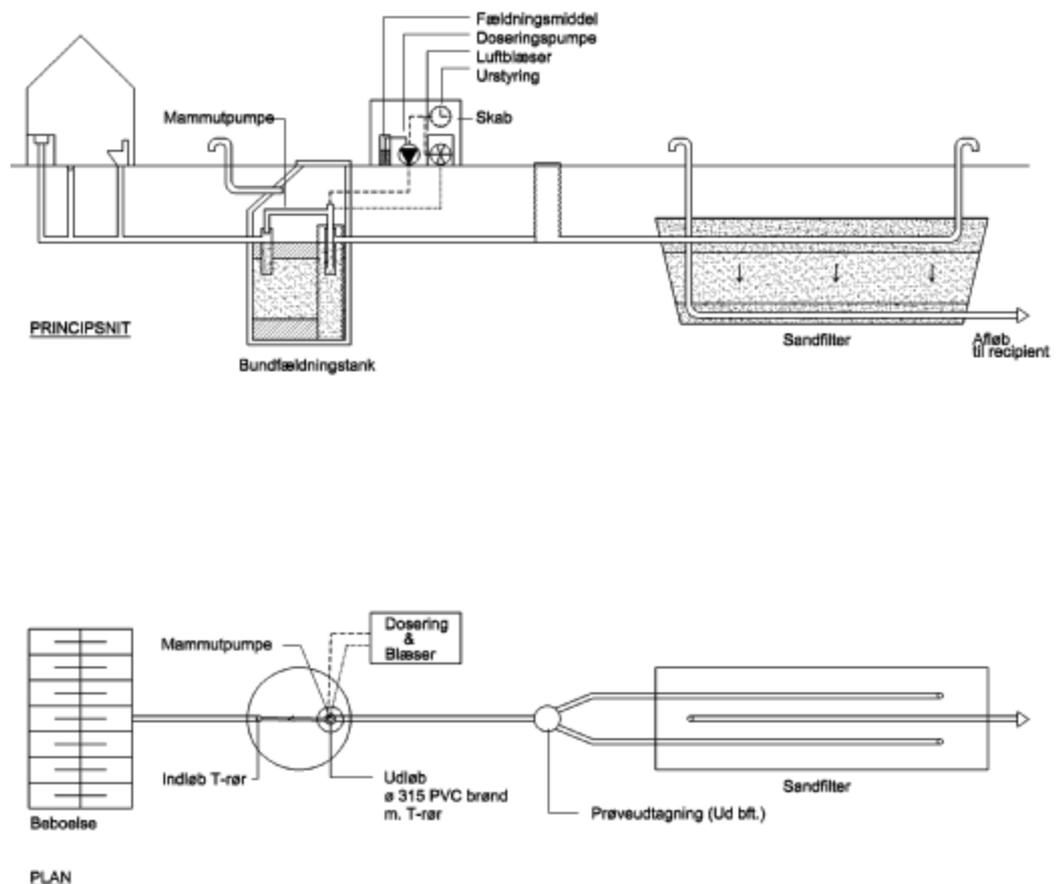
FIGUR 2: ÆLDRE BIOLOGISK SANDFILTER MED GRAVITATION
