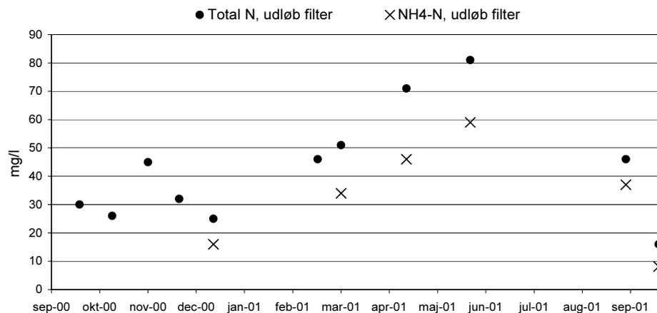
FIGUR 19: KONCENTRATION AF TOTAL-N OG NH<sub>4</sub>-N I UDLØB FRA FILTER.
