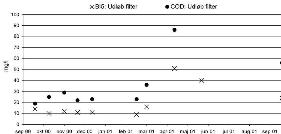
FIGUR 16: KONCENTRATION AF BI<sub>5</sub> OG COD I UDLØB FRA FILTER.
