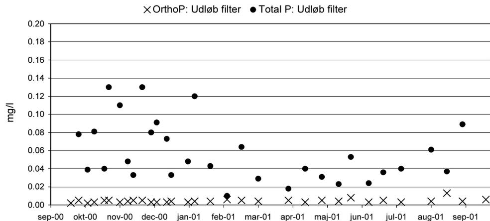
FIGUR 18: KONCENTRATION AF TOTAL P OG ORTHO-P I AFLØB FRA FILTER.
