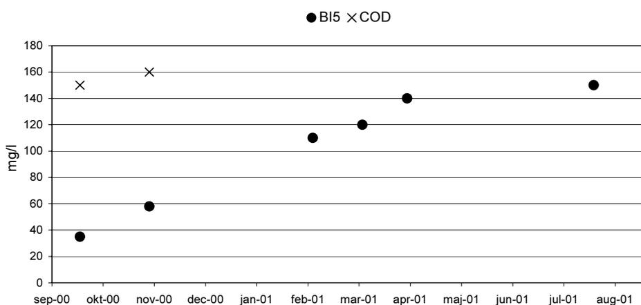
FIGUR 11: KONCENTRATION AF BI<sub>5</sub> OG COD I UDLØB FRA BUNDFÆLDNINGSTANK.
