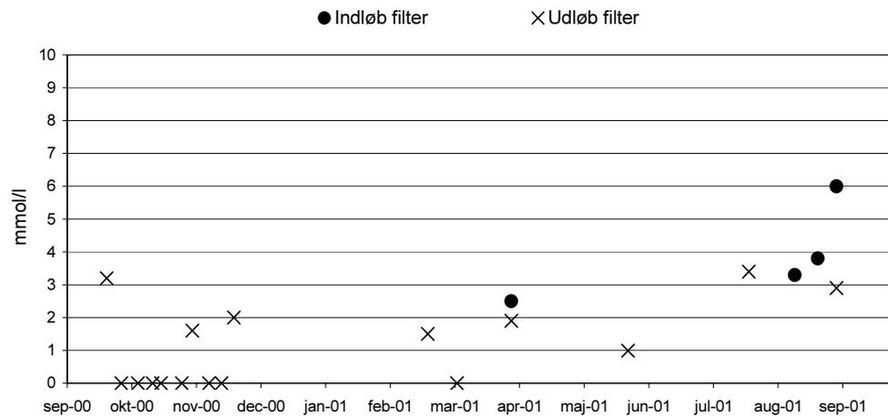
FIGUR 9: ALKALINITET IND OG UD AF SANDFILTER.
