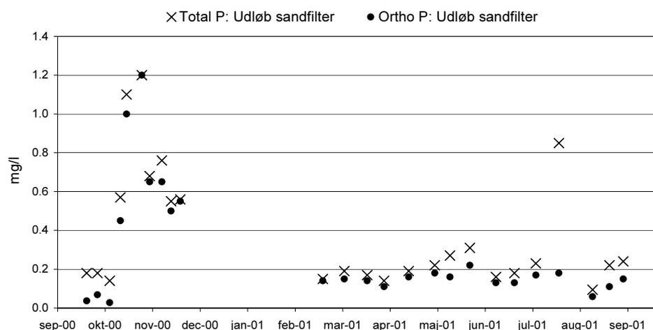
FIGUR 5: UDLØBSKONCENTRATION AF TOTAL FOSFOR OG ORTHO-P FRA SANDFILTER.
