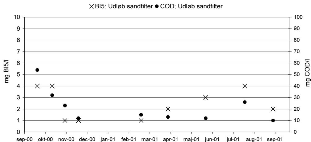
FIGUR 4: UDLØBSKONCENTRATION AF BI<sub>5</sub> OG COD FRA SANDFILTER.
