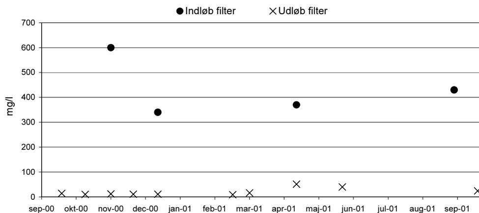
FIGUR 17: KONCENTRATION AF BI<sub>5</sub> I IND- OG UDLØB FRA FILTER.
