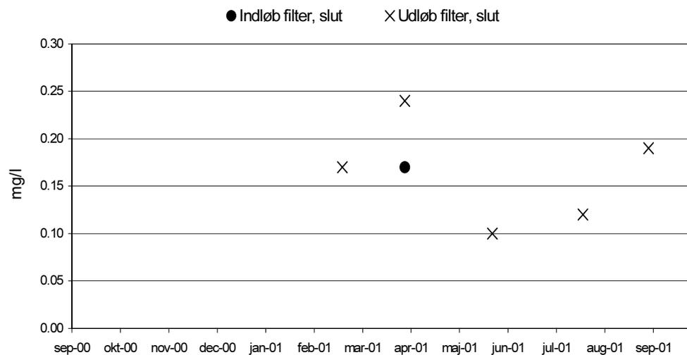
FIGUR 10: KONCENTRATION AF ALUMINIUM IND OG UD AF SANDFILTER.
