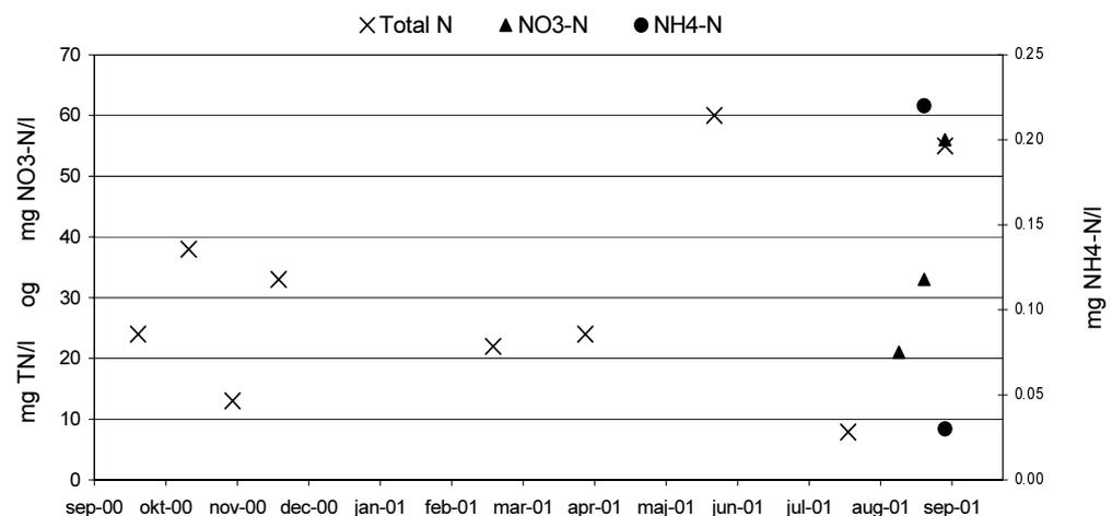
FIGUR 6: UDLØBSKONCENTRATION AF TOTAL-N, NH<sub>4</sub>-N OG NH<sub>3</sub>-N FRA SANDFILTER.
